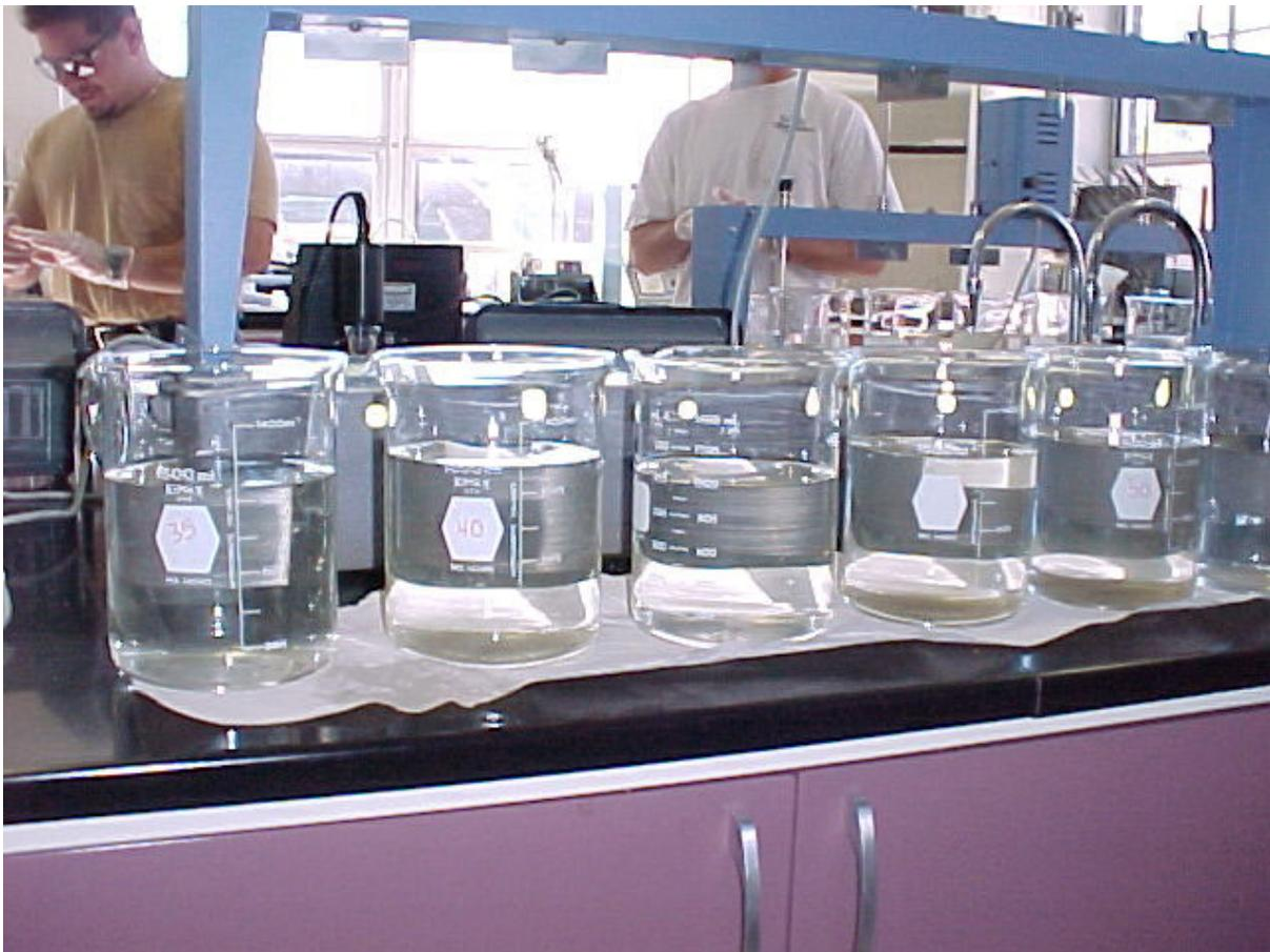
Jar testing is used to determine what chemical dosage is best.
