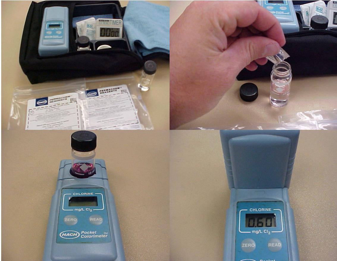
Small portable chlorine measuring kit. The redder the mixture, the hotter or stronger the chlorine is in solution.
