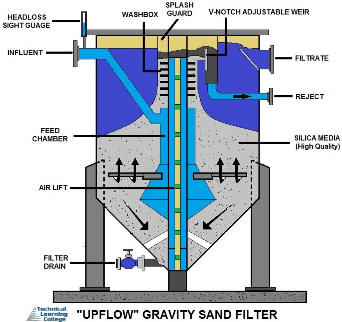
The "Upflow" gravity sand filter, also known for continuous backwashing of the media, is used for many applications such as water treatment and tertiary treatment. This process aids in the removal of inorganic and organic contaminants.
