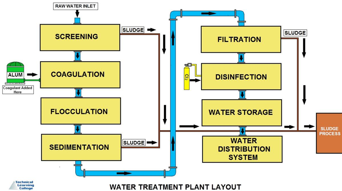
The design of a water treatment plant is determined by the water quality characteristics. Conventional water treatment plants include the steps as shown above if the quality of the source water is variable or poor. Direct filtration plants do not require sedimentation because the water quality characteristics are better.
