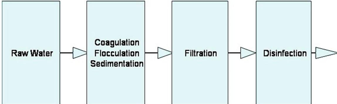
Suspended particles carry an electrical charge which causes them to repel one another. The conventional process uses alum (aluminum sulfate or ferric chloride) and cationic polymer to neutralize the charge. That allows suspended particles to clump together to form more easily filtered particles.
