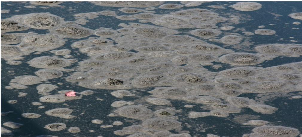
The above photo shows clumps formed by Powder Activated Carbon.
