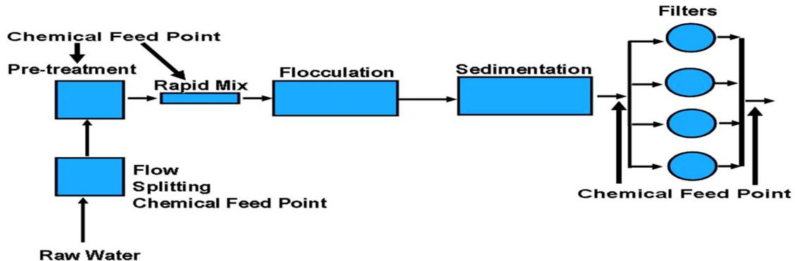
The filter used in the filtration process can be compared to a sieve or microstrainer that traps suspended material between the grains of filter media. However, since most suspended particles can easily pass through the spaces between the grains of the filter media, straining is the least important process in filtration.
