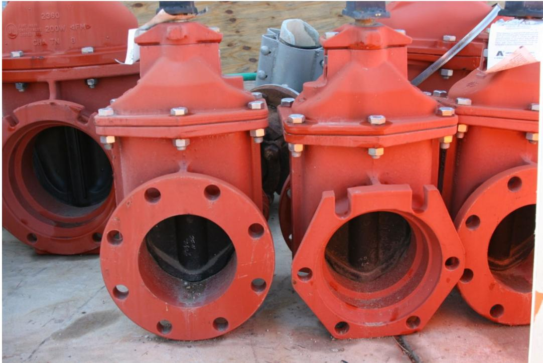
Gate valve storage procedures. Always store a gate valve with the gate up or opened. Not like this photograph. Sunlight destroys the rubbers with ultraviolet radiation. Dr. Rusty recommends that you keep the valves covered and clean. We are professionals and must remember the final outcome. We provide drinking water to the public. Notice the two different styles of flange fittings.
