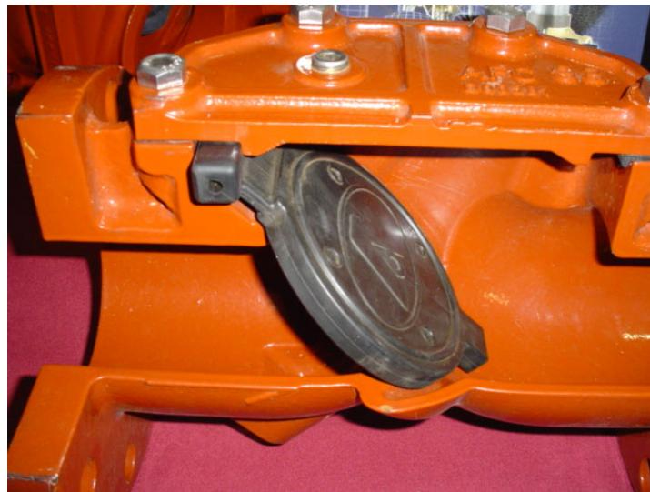
A beautiful swing check valve. Swing checks need to be maintained. I hate finding a swing check that is both buried and forgotten, rusted in place or, my favorite, the check was removed.
