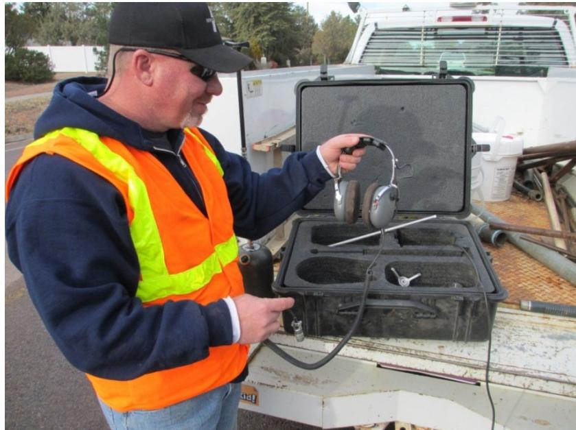
Leak detection is critical for finding difficult to locate leaks. There are many devices to choose from. All of these devices magnify the sound of the leak to pin-point the area of damage. Plastic pipe is the most difficult and copper is the easiest to locate.
