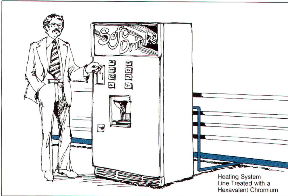
Several cross-connections have been made to soda machines, the one to worry about is when you have a copper water line hooked to CO<sub>2</sub> without a backflow preventer.
