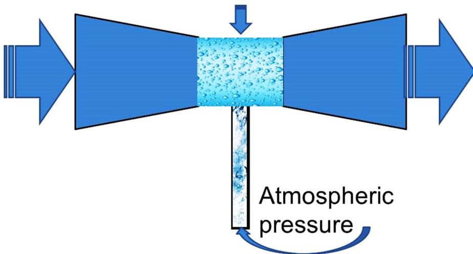
The newest injector design causes complete mixing of injected materials (air, ozone or chemicals), eliminating the need for other in-line mixers. Venturi injectors have no moving parts and are maintenance free. They operate effectively over a wide range of pressures (from 1 to 250 psi) and require only a minimum pressure difference to initiate the vacuum at the suction part. Venturis are often built in thermoplastics (PVC, PE, PVDF), stainless steel or other metals.
