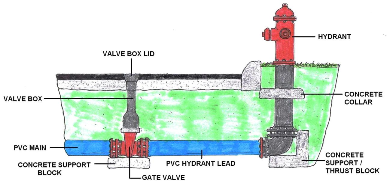
The above diagram is for proper fire hydrant and isolating gate valve installation. The diagram below represents how rust and electrolysis creates a hole or break in iron based water mains.
