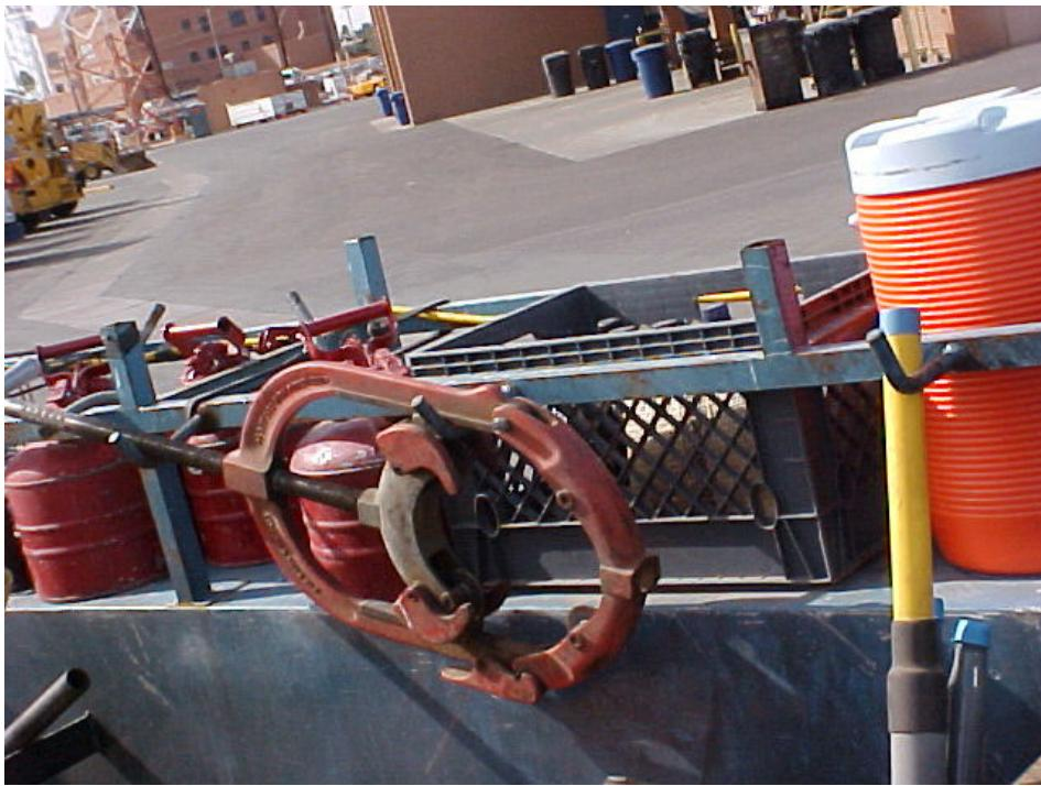
Here is a four-way pipe cutting tool used for iron pipe. Be careful not to break the wheels by over-tightening. I personally like 4-Ways because of the nice cut. You will learn to recognize the distinct snap of cut pipe. The only drawback to these cutters is cutting a small section out of the main.
