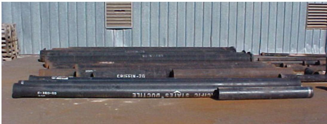
**Ductile pipe cement-lined iron pipe.** I've seen thousands of dollars of pipe that is dropped or moved with the front bucket of a backhoe and destroyed. This destroys the interior protection of the pipe, causing leaks which will start within a short period of time, just a few years. I know that some of you welcome this as job security. Always protect and store all types of pipe covered and in a pipe rack. This goes for the proper storage of rubbers as well.
