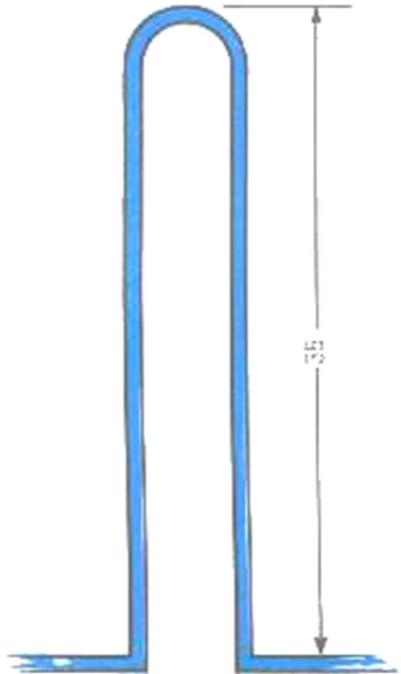
Gauge pressure is simply the pressure read on the gauge. If there is no pressure on the gauge other than atmospheric, the gauge will read zero. Then the absolute pressure would be equal to 14.7 psi, which is the atmospheric pressure.
