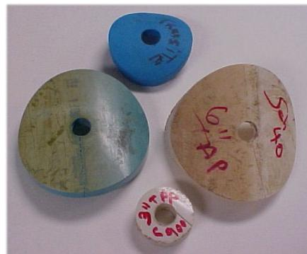
Various types and sizes of coupons or tap cut-outs. You will want to date and collect these cut-outs to determine the condition of the pipe or measure the corrosion.
