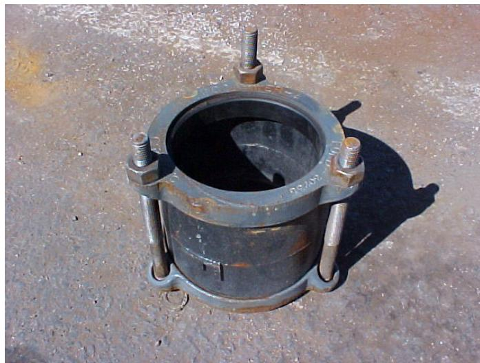
**Flex Coupling**--sometimes referred to as a Dayton; used to join pipes or to "cut-in a valve." You will learn that you can use different sizes to join pipe or even file out the inside diameter to adjust to larger pipes like ACP. This flex coupling only has three bolts. I like four or more for work with larger pipe work.
