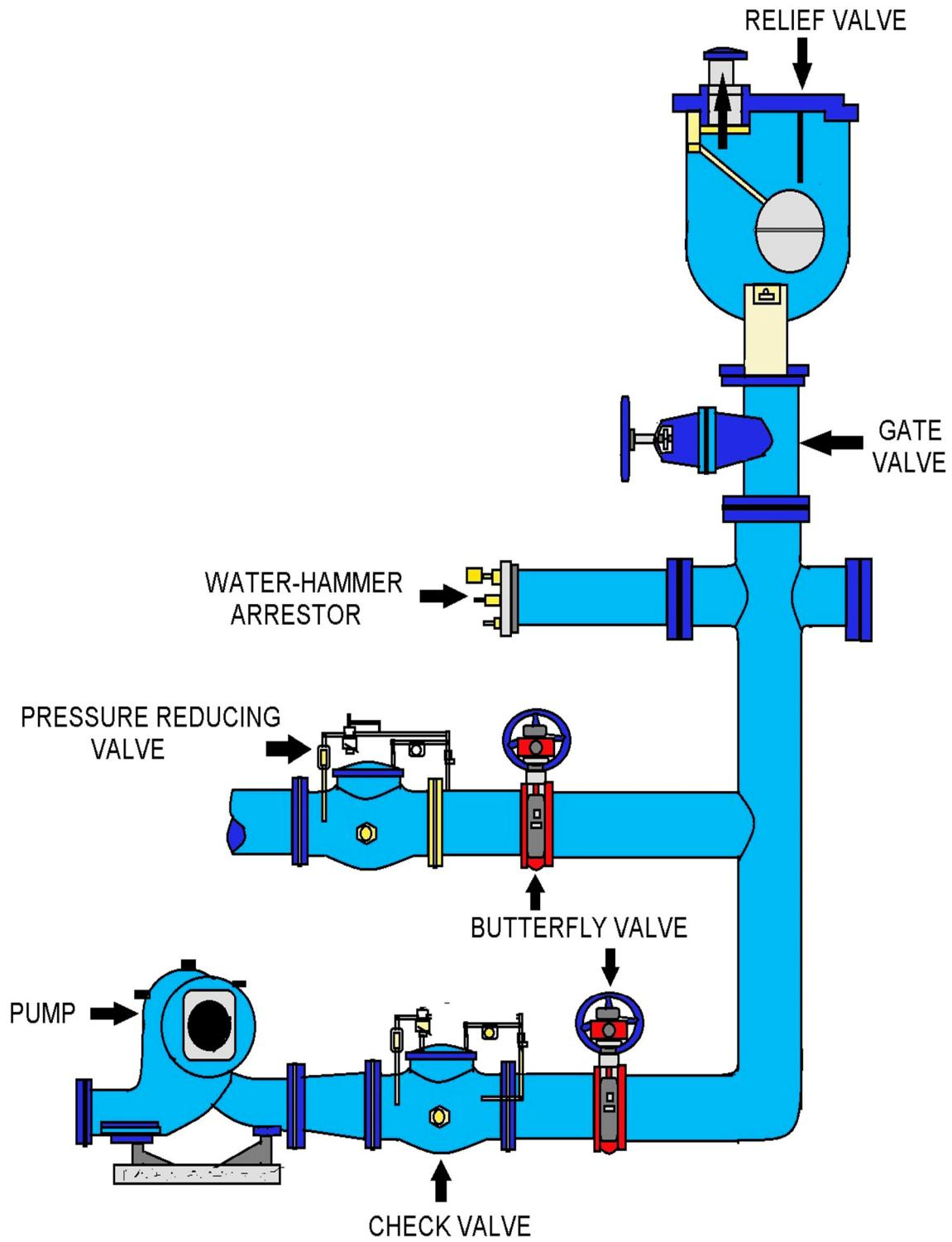
**AIR RELIEF VALVE INSTALLATION DIAGRAM**
