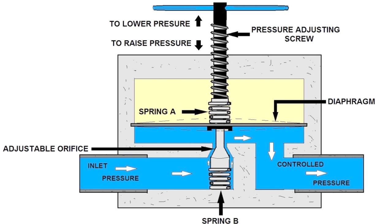
**PRESSURE – REGULATION VALVE DIAGRAM**
