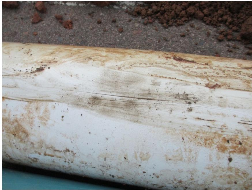
Generally speaking, water main breaks are much more intense than service leaks. This scenario will examine a hairline crack caused by poor installation. The water main was laid on a sharp rock without proper bedding. A slight water main leak is often confused with a service line leak and can be difficult to find.
