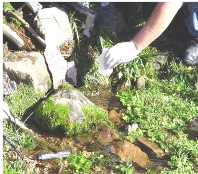
Sampling downstream from a wastewater plant's discharge point.
