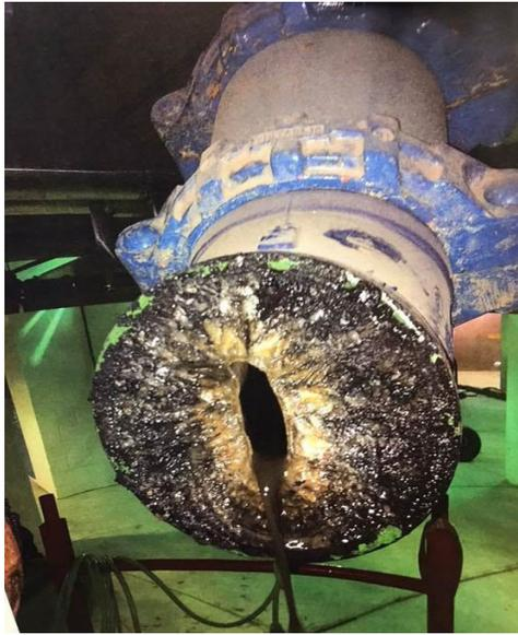
Struvite deposits inside a digester pipe.
