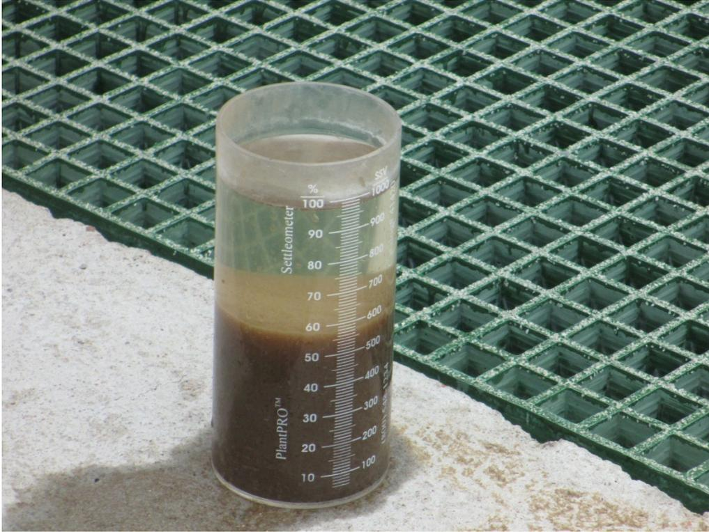
The settleometer is a great tool for operators. It indicates how the solids will settle in the clarifier and the density of the sludge.
