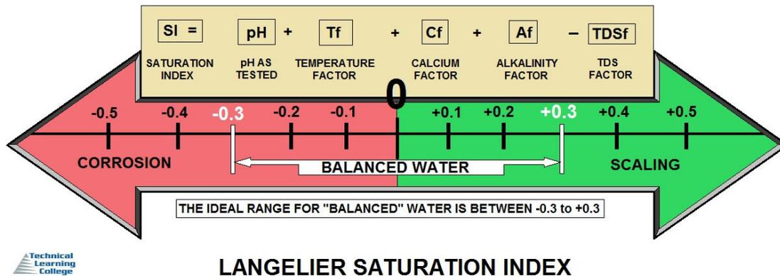
Water with a Langelier saturation index of 1.0 is one pH unit above saturation. Reducing the pH by 1 unit will bring the water into equilibrium. This occurs because the portion of total alkalinity present as  $\text{CO}_3^{2-}$  decreases as the pH decreases, according to the equilibria describing the dissociation of carbonic acid:
