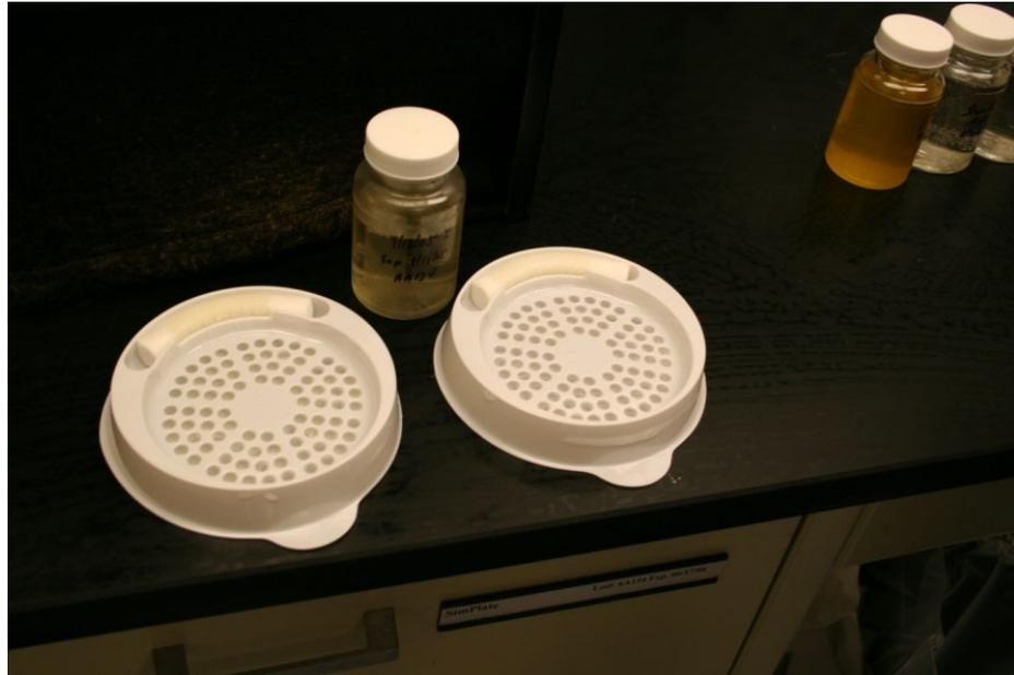
IDEXX's SimPlate for HPC method is used for the quantification of heterotrophic plate count (HPC) in water.
