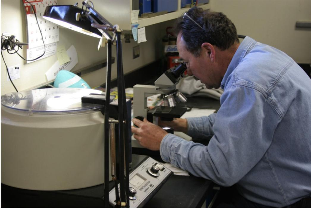
Phase microscopes are used to see indicator bugs and other MO's microorganisms. This examination is used so that the operator knows how well the process is working.
