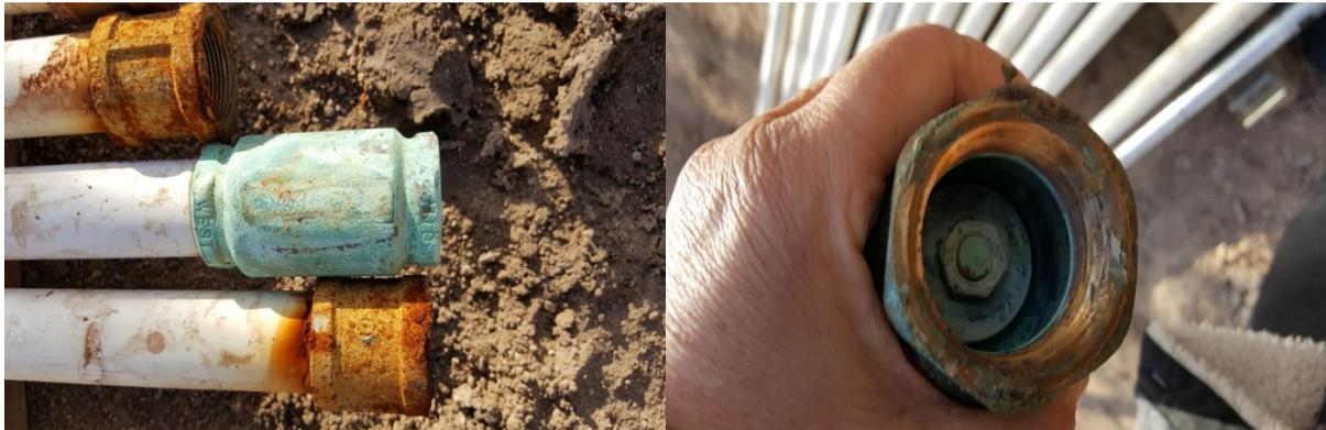
It is recommended to install a check valve every 100 feet of piping. Sometimes the valve becomes defective and causes pumping issues. When installing the the check valve, the correct direction of the check valve is important.
