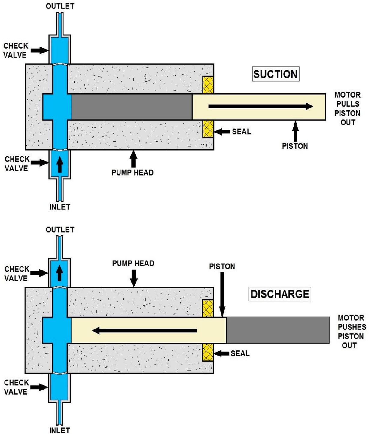
**POSITIVE DISPLACEMENT PUMP DIAGRAM
