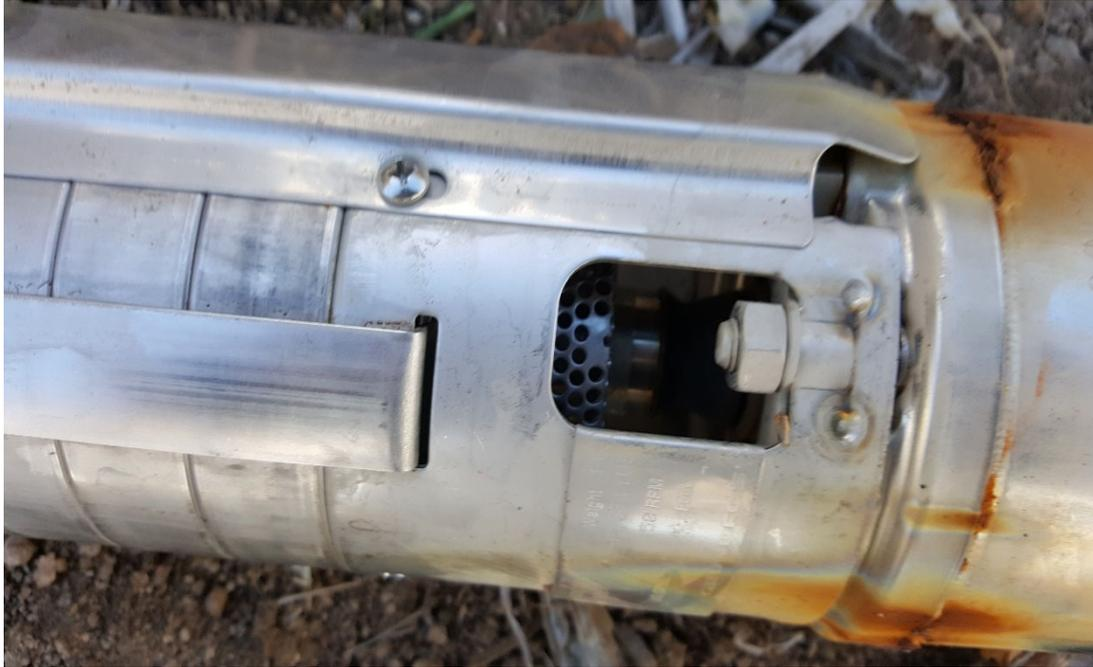
Pump and motor connection.
