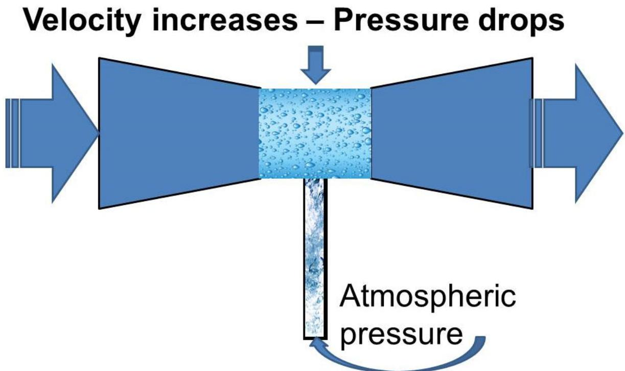
The newest injector design causes complete mixing of injected materials (air, ozone or chemicals), eliminating the need for other in-line mixers. Venturi injectors have no moving parts and are maintenance free. They operate effectively over a wide range of pressures (from 1 to 250 psi) and require only a minimum pressure difference to initiate the vacuum at the suction part. Venturis are often built in thermoplastics (PVC, PE, PVDF), stainless steel or other metals.
