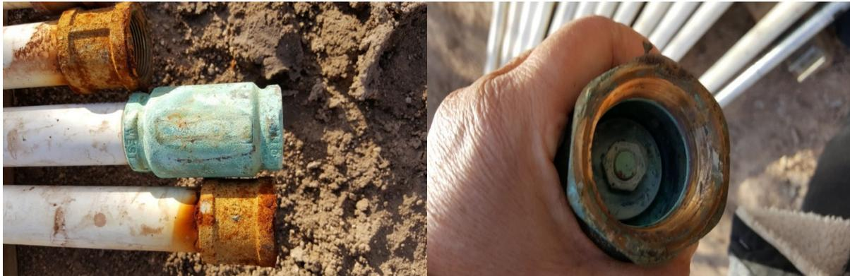
It is recommended to install a check valve every 100 feet of piping. Sometimes the valve becomes defective and causes pumping issues. When installing the the check valve, the correct direction of the check valve is important.
