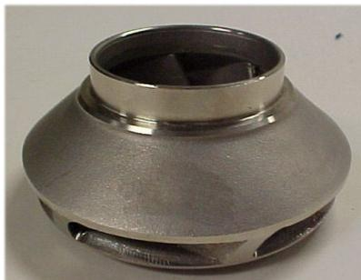
Closed Pump Impeller
