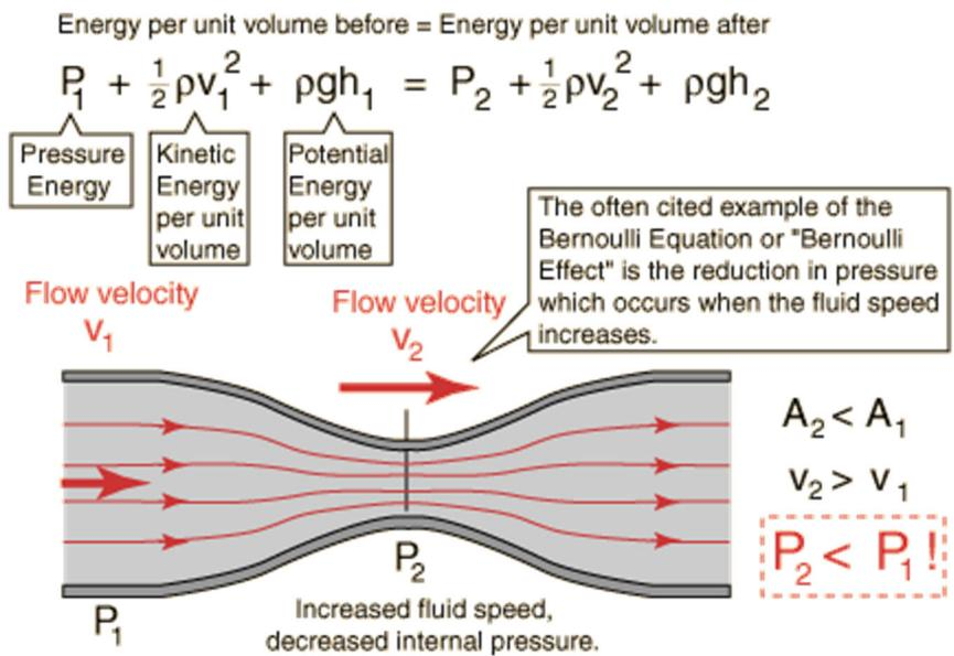
A special form of the Euler's equation derived along a fluid flow streamline is often called the **Bernoulli Equation**.
