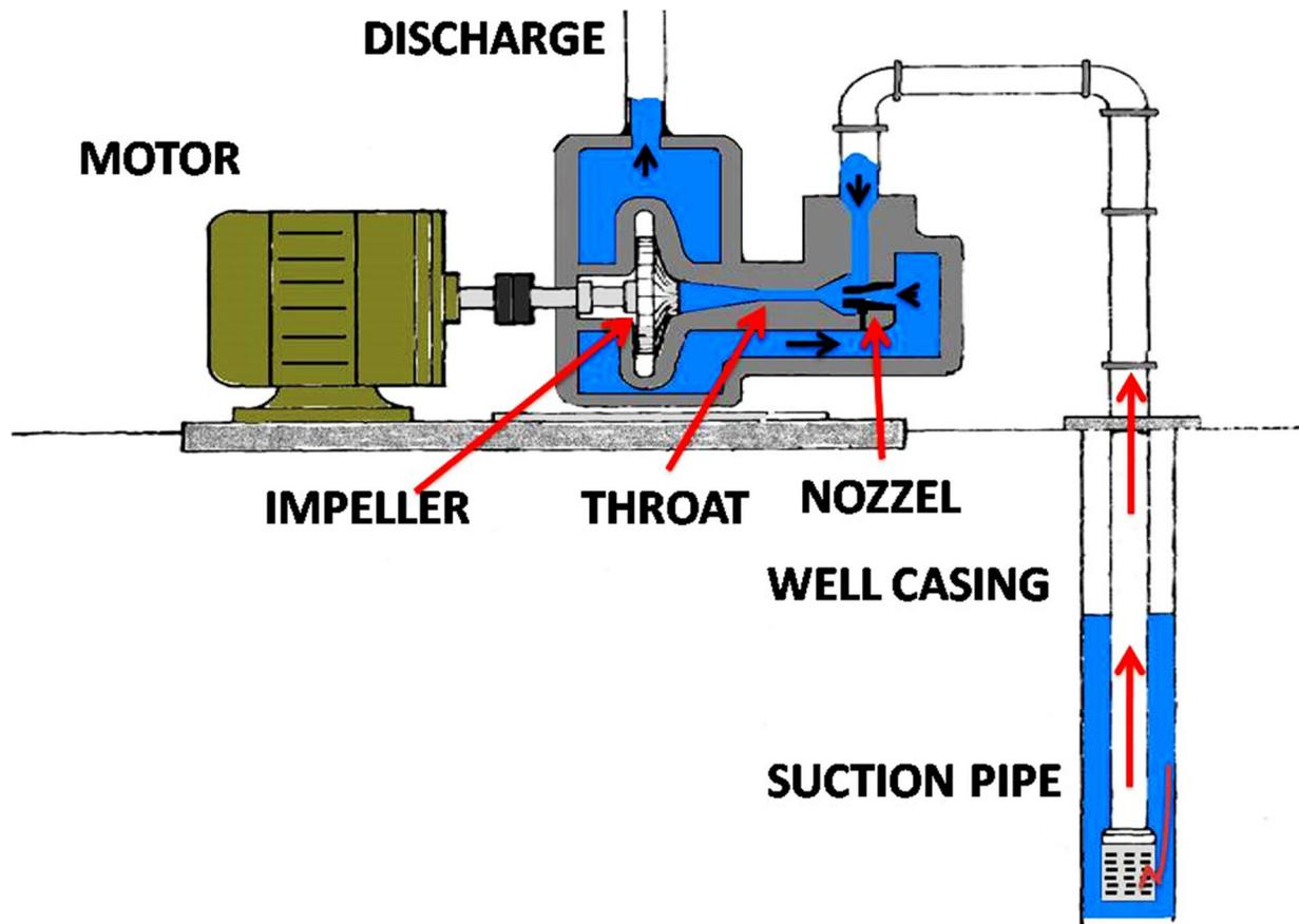
**SUBMERSIBLE PUMP WITH BOOSTER DIAGRAM #2**
