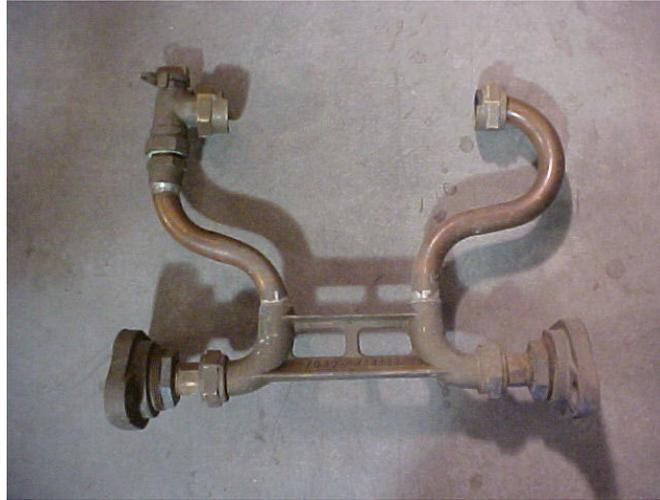
Water Meter Re-setter, Riser, or sometimes referred to as a copper yoke. There is also a cast iron version which is best broken off with two sledge or cocking hammers when it's time to replace or retrofit the service. You almost always replace a yoke stop hot. A Yoke stop is an Angle Stop most of the time but I've seen a nasty galvanized valve that is also used in this situation.
