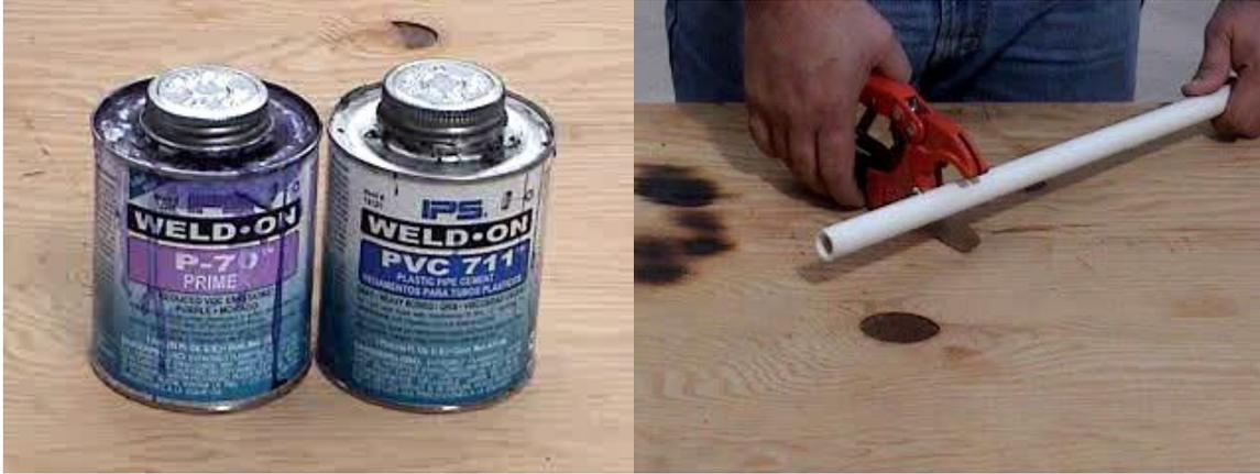
Solvent Cementing is the most popular kind of CPVC joining method. Remember, always wear eye protection and gloves.
