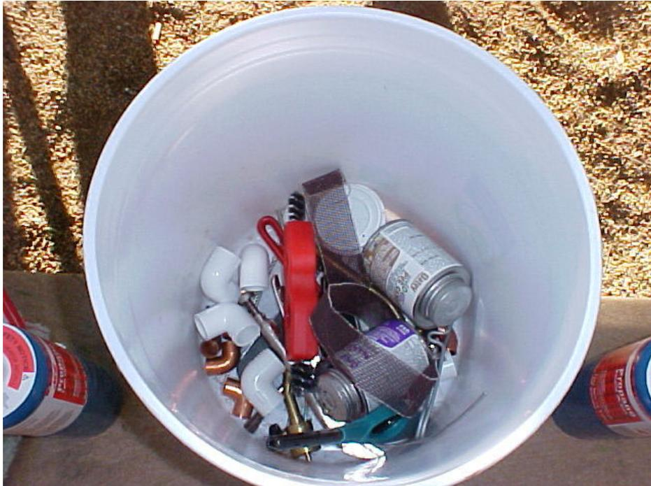
Commonly found materials used for sweating (Soldering) copper pipe and gluing (Cementing) PVC. Plumbers like to utilize 5-gallon buckets as a tool box of sorts.
