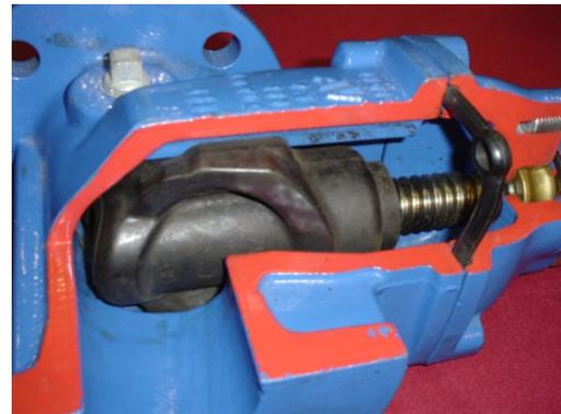
The gate is usually wedge-shaped. When the valve is wide open the gate is fully drawn up into the valve bonnet. This leaves an opening for flow through the valve the same size as the pipe in which the valve is installed.
