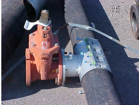
Gate Valves are used to isolate sections of water mains. Not to be used to throttle or regulate the flow.
