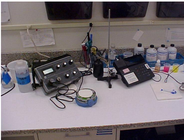
Commonly found conductivity, temperature and pH measuring equipment. As a sampler, you will use this equipment on a daily basis. Make sure to date the pH buffers and calibrate your equipment every morning.
