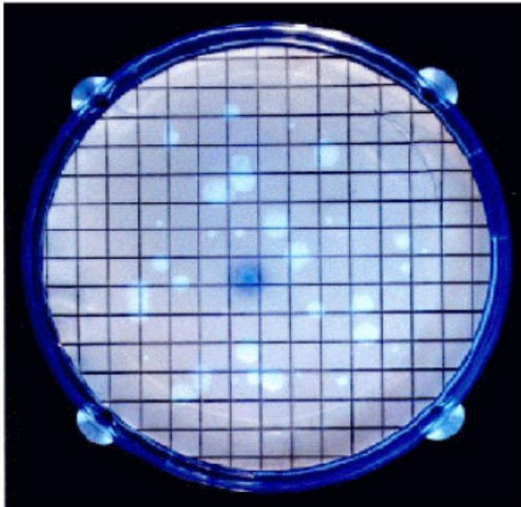
**Figure 1.** This photograph shows *Escherichia coli* (blue/green fluorescence) and total coliforms other than *E. coli* (blue/white fluorescence) on MI agar under long wave UV light (366 nm). The sample used was a wastewater-spiked Cincinnati, Ohio tap water.
