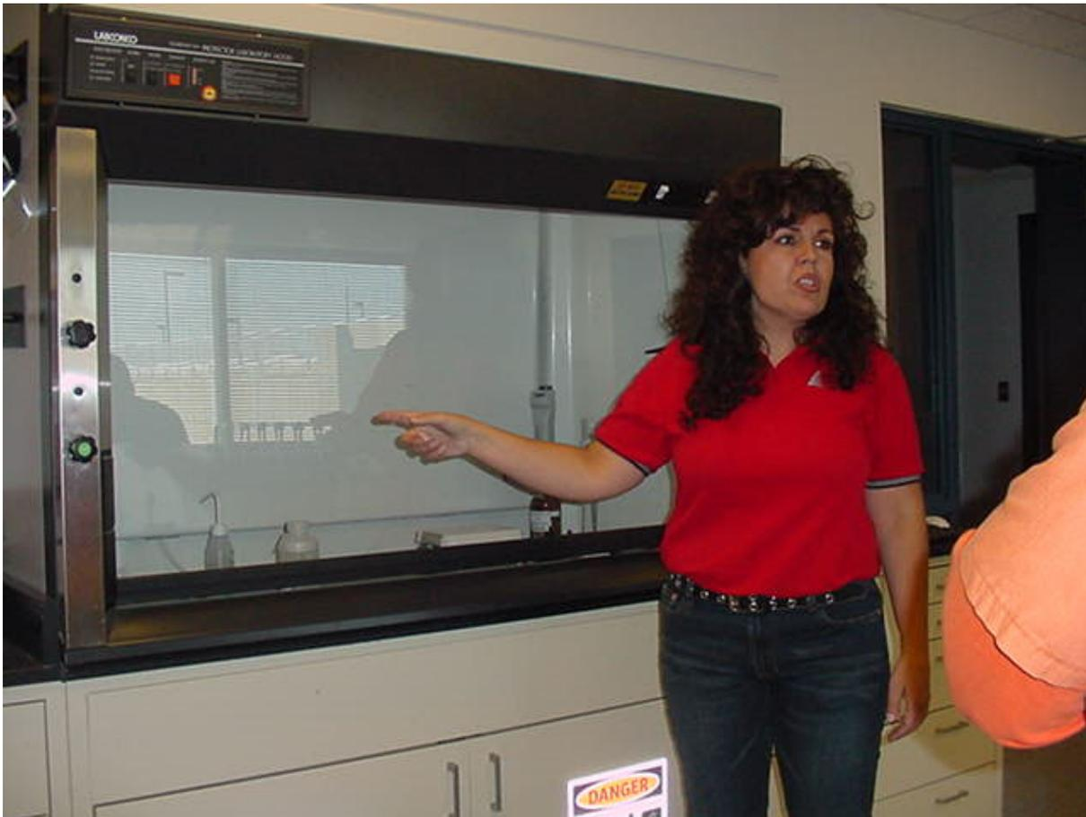
Always utilize a chemical fume hood and ventilation system when working or testing Chlorine. Melissa Durbin shown in photo.
