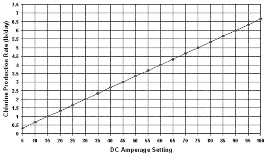
**Note:** With time, the membrane accumulates calcium and other mineral deposits that increase the resistance between the electrodes. The increased resistance causes a reduced amperage output and a corresponding reduced chlorine output. The system needs periodic membrane cleaning to recover the desired amperage output. A water softener system can be added to the system water supply to reduce the amount of calcium, thus increasing the service life of the membrane.
