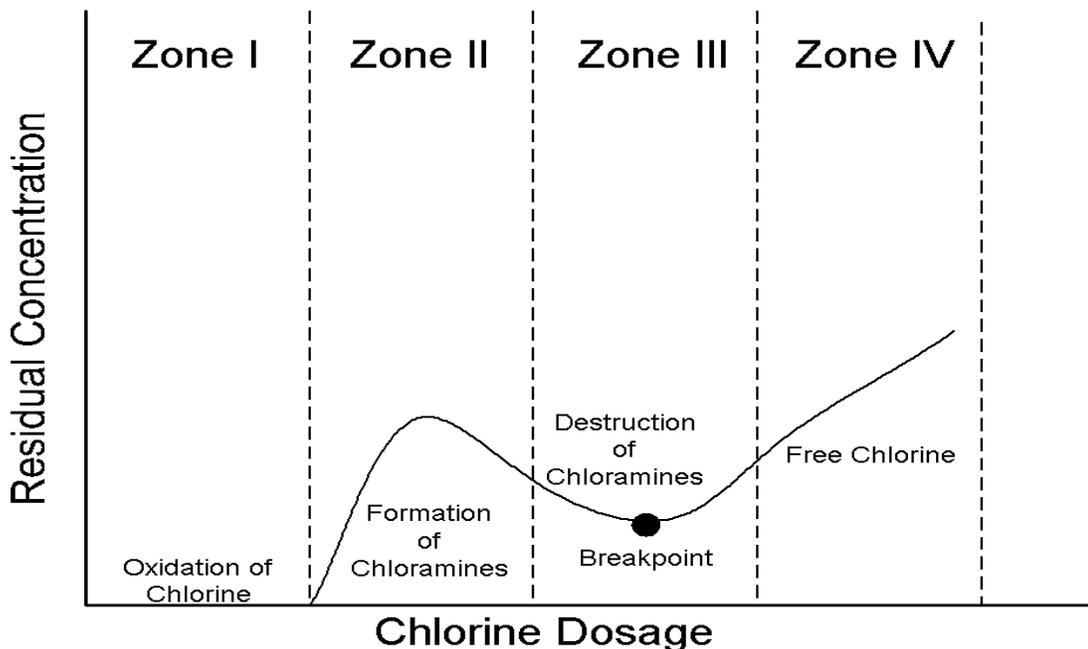
The graph shown depicts the chlorine residual as a function of increasing chlorine dosage with descriptions of each zone given below (Drawing by Erik Johnston, adapted from Reynolds and Richards, 1996).
