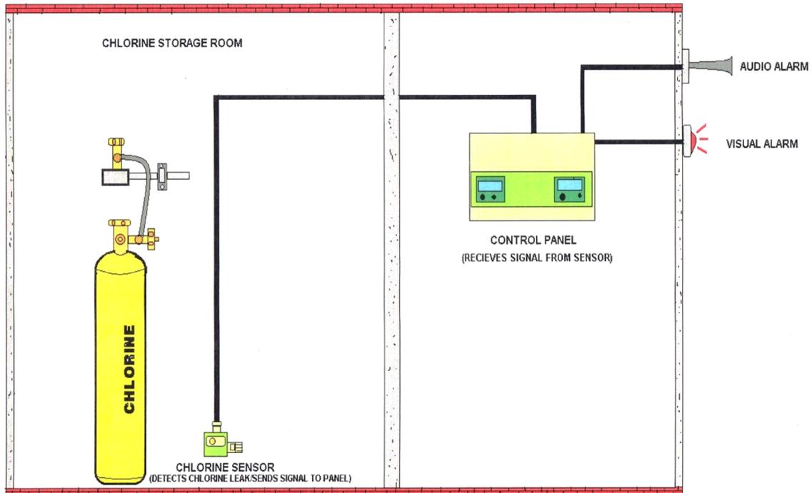
For all treatment facilities, chlorine gas under pressure shall not be permitted outside the chlorine room. A chlorine room is where chlorine gas cylinders and/or ton containers are stored. Vacuum regulators shall also be located inside the chlorine room. The chlorinator, which is the mechanical gas proportioning equipment, may or may not be located inside the chlorine room.
