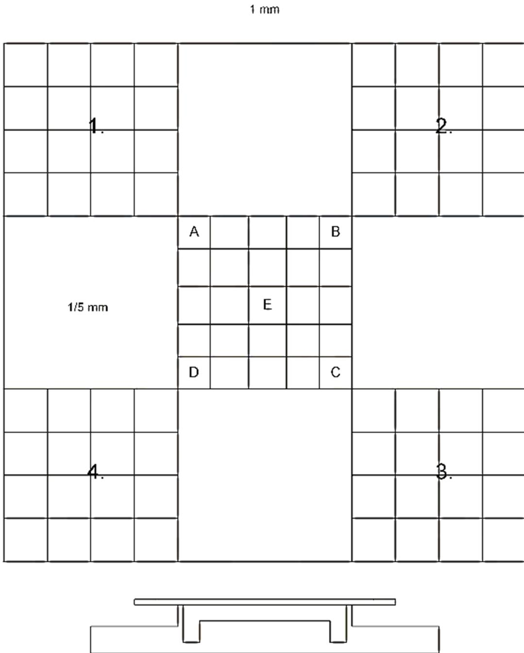
**Hemacytometer Platform Ruling. Squares 1, 2, 3, and 4 are used to count stock suspensions of *Cryptosporidium* oocysts and *Giardia* cysts (after Miale, 1967)**
