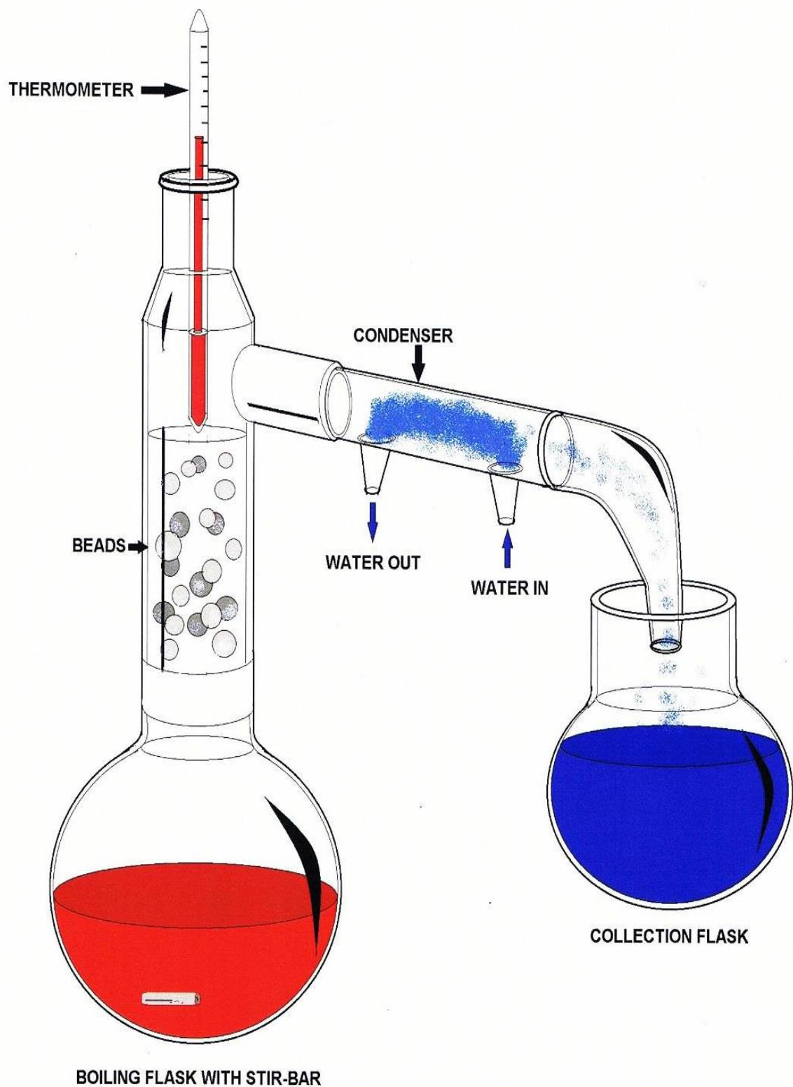
BOILING FLASK WITH STIR-BAR
