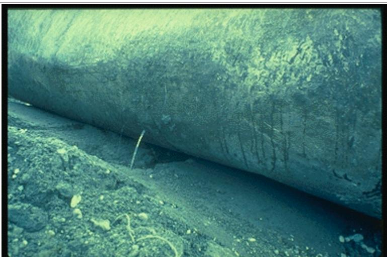
Water(?) leaking from a hole in the side of a freshly excavated UST.
