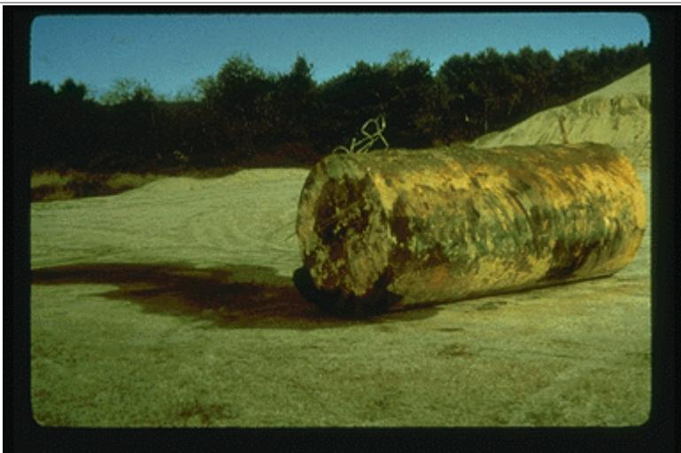
Product leaking from holes in a freshly excavated UST.
