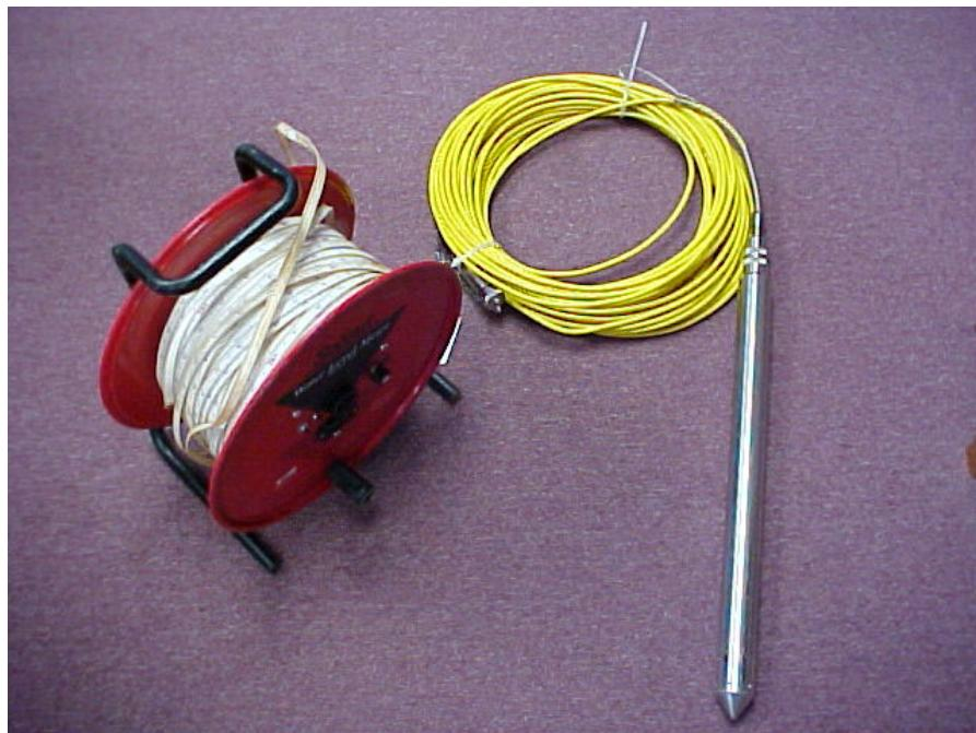
Groundwater Transducer (pH, Temp. chemical detection, and D.O.) and depth probe. These tools are used to find the depth and pH of well water.
