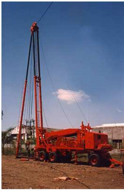
Typical Cable Tool Rig
