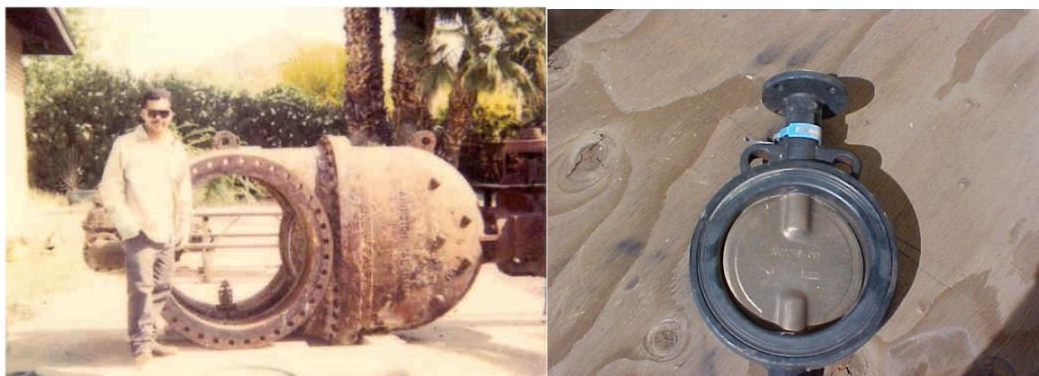
Large Gate Valve and a Butterfly Valve which works like an old fashioned carburetor.
