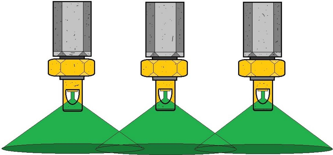
**FLAT FAN NOZZLE WITH PROPER PATTERN OVERLAP
