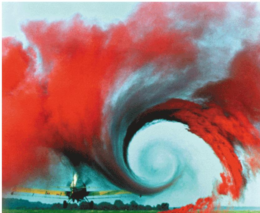
NASA's Langley Research Center performed a number of wake vortex studies at its Wallops Island facility. A crop duster was flown low and slow over a red smoke flare. As the wing tip passed over the smoke generator, the vortex created a turbulent flow that can cause control problems to following aircraft. *Image: NASA*
