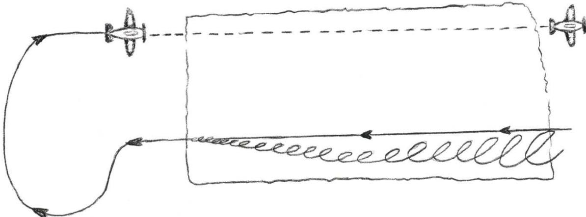
When this fits in with crop rows, the pilot can line up the aircraft with a crop row. If the area is too rugged or steep for these patterns, flight lines should follow along the contours of the slopes. Where spot areas are too steep for contour work (mountainous terrain), make all treatments down slope. Avoid flying parallel to a stream or large lake if there is a tendency for drift toward the stream or lake.
