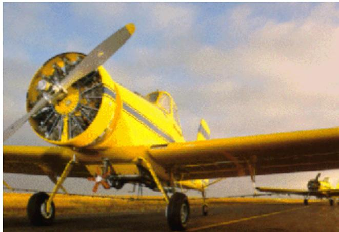
The AT-401B is a 400 gallon workhorse powered by the Pratt & Whitney R-1340 radial engine. It incorporates all the rugged durability, safety features, and flying ease that Air Tractors are known for with the low price tag of a piston engine plane.
