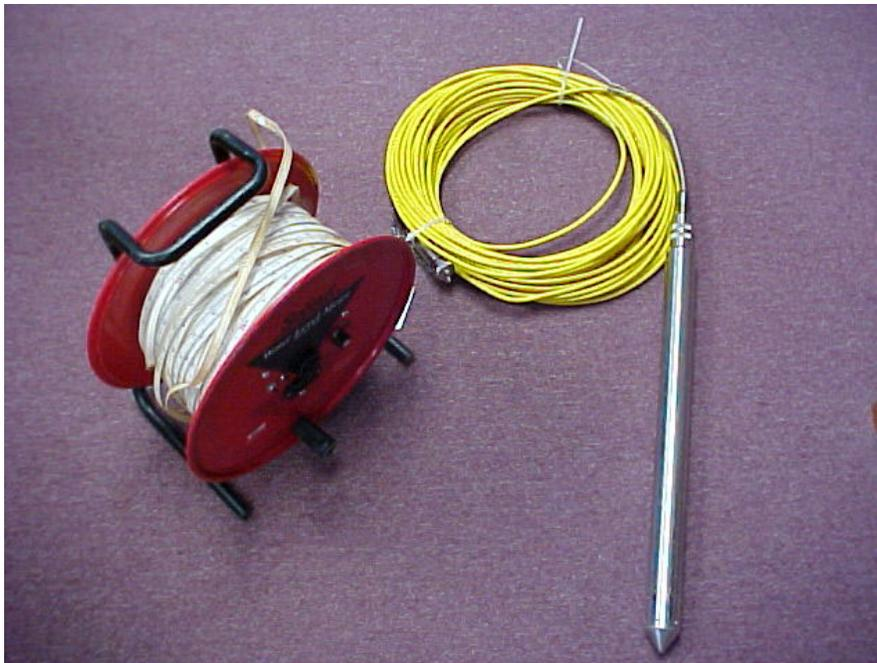
Groundwater Transducer (pH, Temp. chemical detection and D.O.) depth probe. These tools are used to find the depth and pH of well water.
