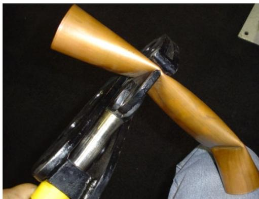
Copper Tubing Crimpers. Great if you are unable to get a shut-down. Just place this dude on the pipe. The problem is to fix that crimp when you are finished with the leak. They need to invent an uncrimper.
