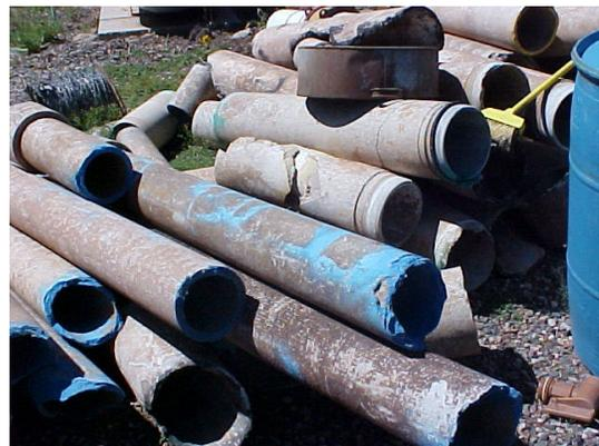
Asbestos is considered a hazardous material, and precautionary measures must be taken to protect water utility workers when cutting, tapping or otherwise handling this type of pipe.
