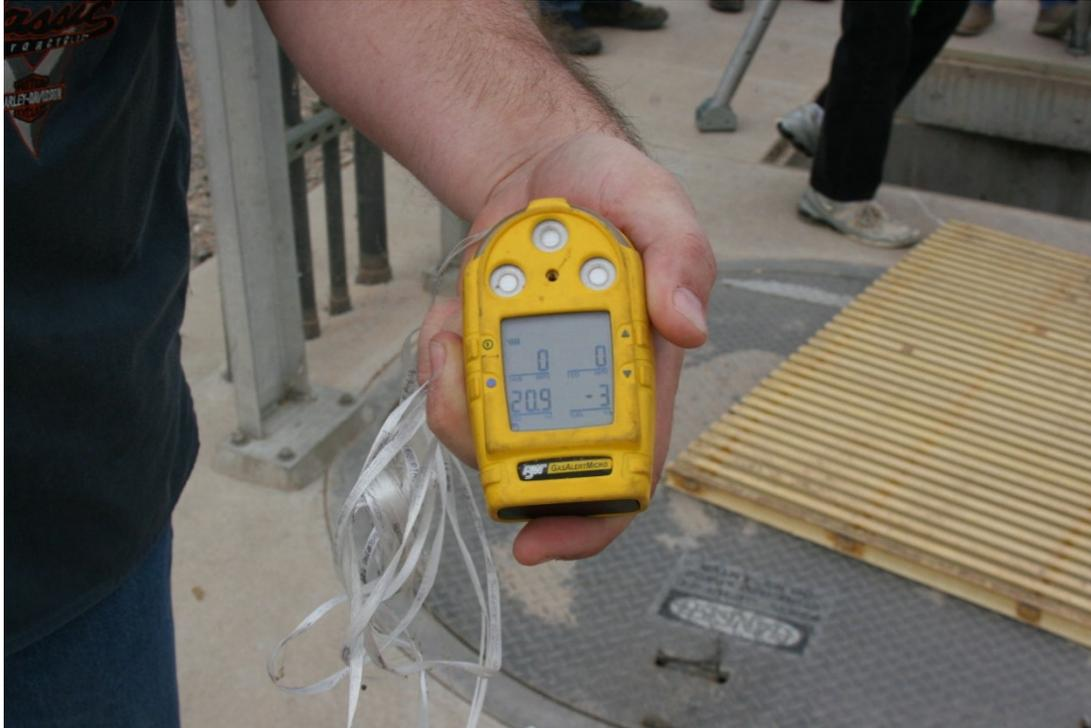
Here is a small clip-on style multi-purpose gas meter. We tied a string to lower the meter in the confined space to get a gas reading before entering.
