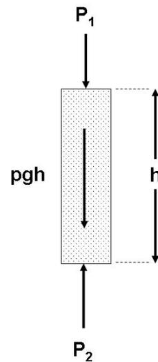
The diagram illustrates the equality of pressures in orthogonal directions. This can be extended to any direction whatever, so Pascal's Principle is established. This demonstration is similar to the usual one using a triangular prism and considering the forces on the end and lateral faces separately.
