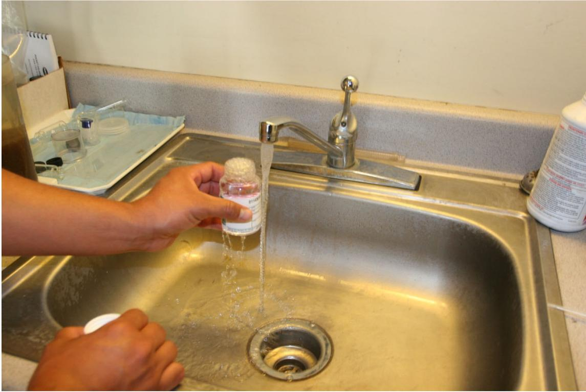
Be careful not to overfill the Bac-T bottle or rapidly fill it. It is easier than you think to contaminate or have a positive sample.
