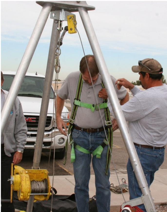
Donning the personal protective equipment (**PPE**) necessary for confined space entry.
