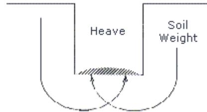
**HEAVING OR SQUEEZING.** Bottom heaving or squeezing is caused by the downward pressure created by the weight of adjoining soil. This pressure causes a bulge in the bottom of the cut, as illustrated in the drawing above. Heaving and squeezing can occur even when shoring or shielding has been properly installed.
