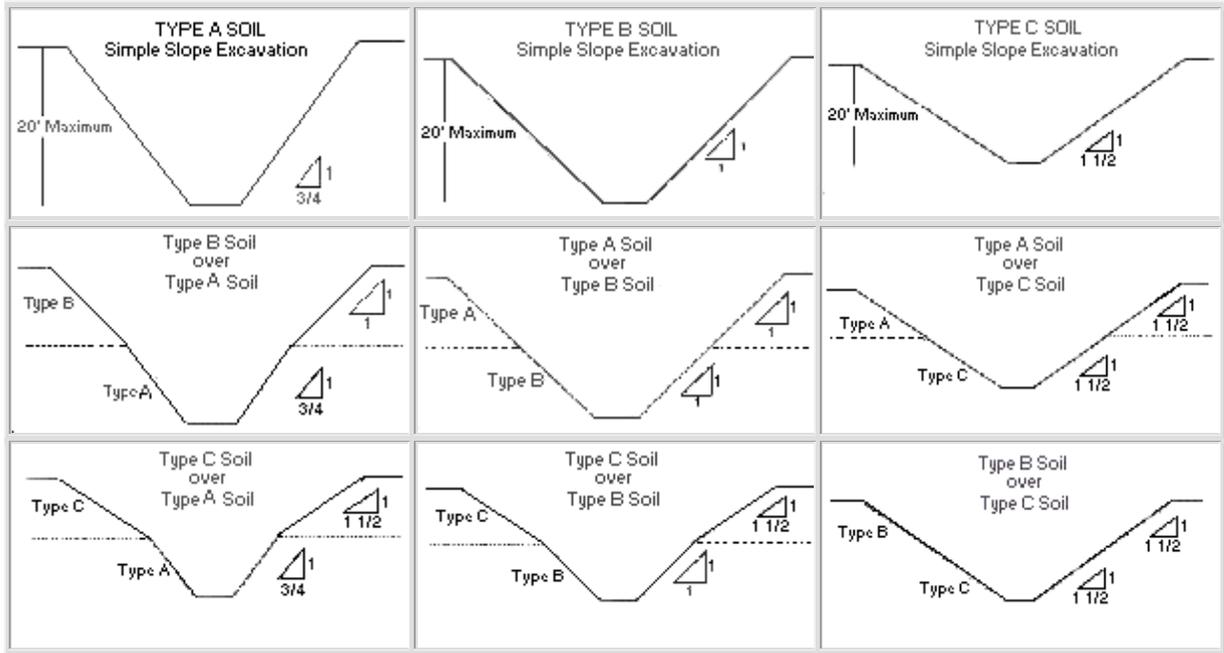
**FIGURE V:2-14. EXCAVATIONS MADE IN TYPE A SOIL.**
