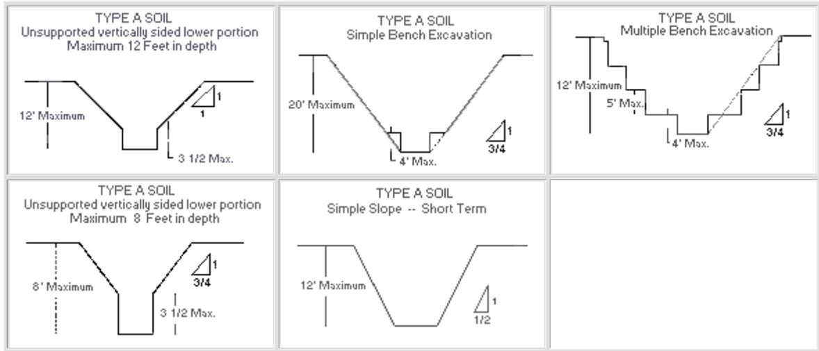
**BENCHING.** There are two basic types of benching, simple and multiple. The type of soil determines the horizontal to vertical ratio of the benched side.
