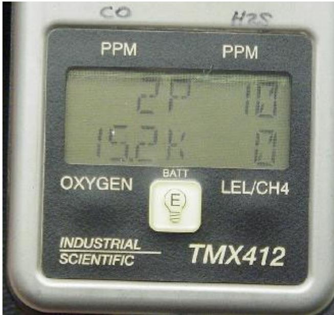
Example Display for Peak Mode: The display reads 2 ppm peak value for CO and 10 ppm peak value for H<sub>2</sub>S (top line); 15.2 % for oxygen and 0 % for LEL (bottom line).
