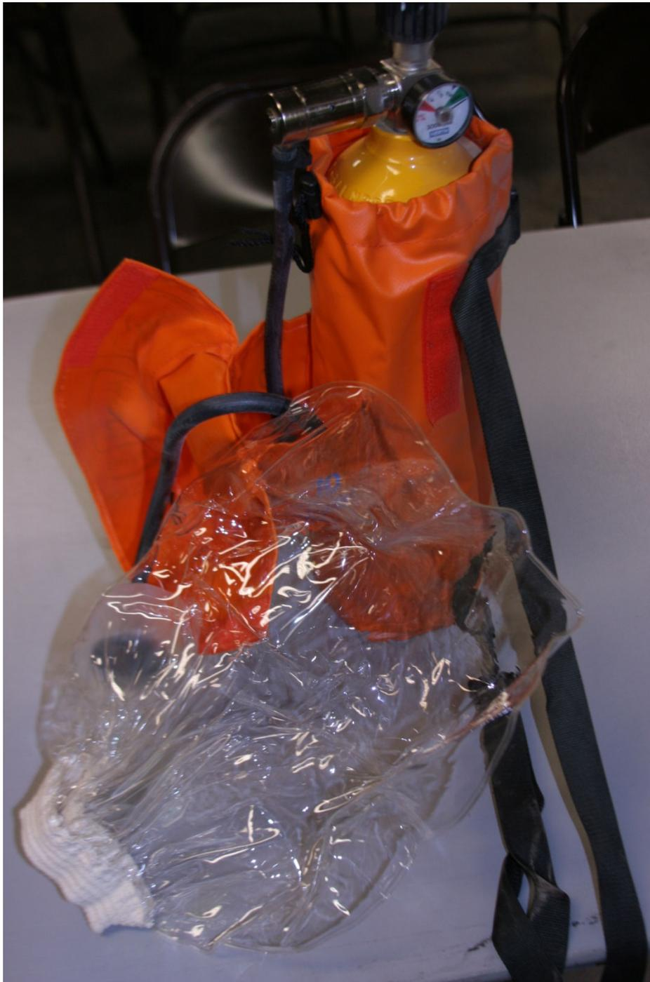
This is a ten-minute escape air pack or emergency air supply. The plastic bag will go over your head during an emergency and provide enough air to get out of the hole. There are smaller versions of this system.
