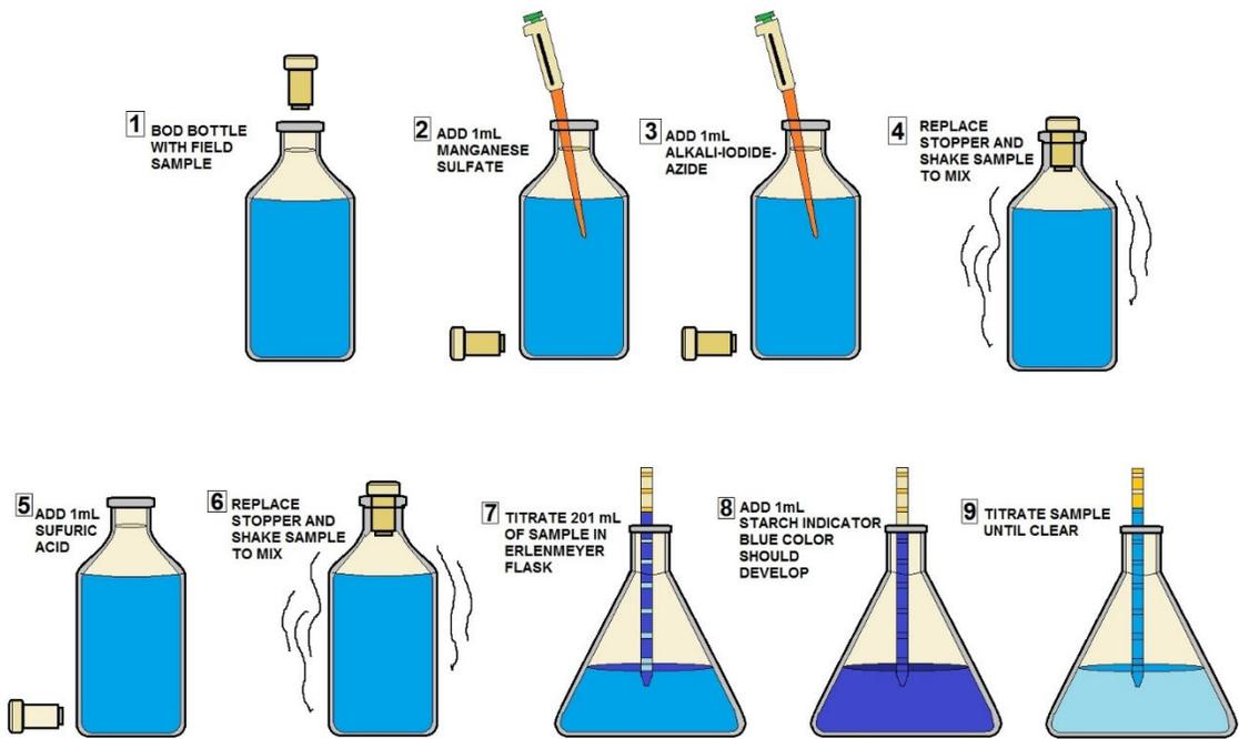
**HOW TO MEASURE DISSOLVED OXYGEN IN A WATER SAMPLE**
