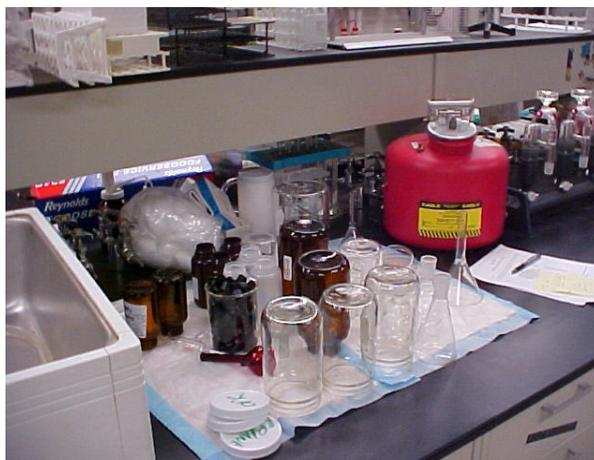
A normal day for a Lab Tech will include the washing of lab glassware. Sometimes the Tech will use acid to wash certain glass bottles. Notice the broken glass or Sharps container.
