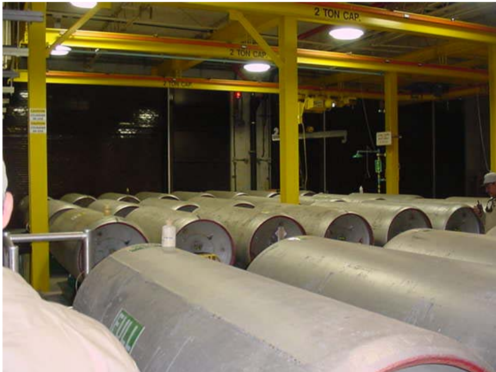
1-ton chlorine gas containers.
