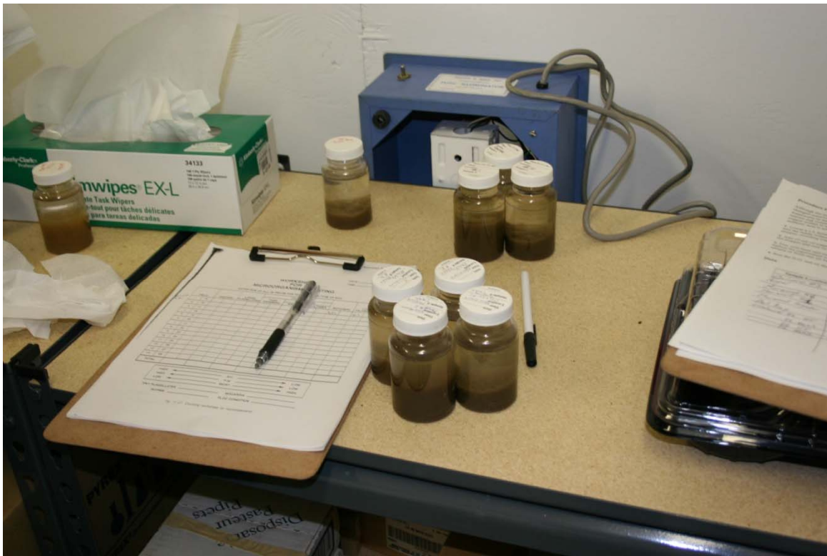
Operators analyze sludge samples to improve wasting.
