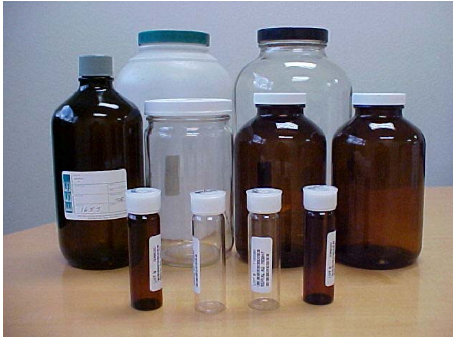
Above, 625/608, 1657, TTO/Organics, TPH/Oil/Grease Smaller bottles-TOCs, VOCs, 601/602 and 502.2.
