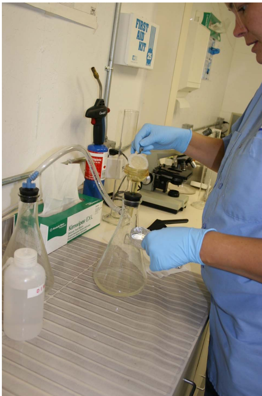
Lab tech removing filter for TSS analysis.
