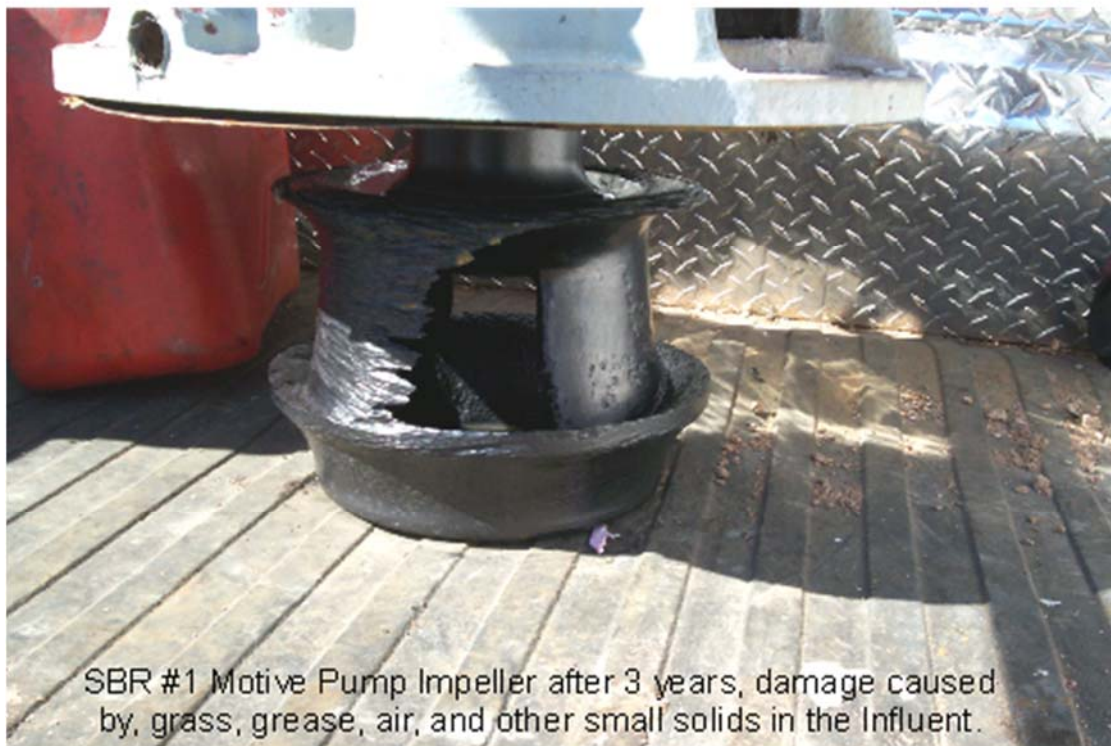
Top photo: Various pump damage from undesirable materials in the sewer system. Bottom photo, heavy grease from not being regularly pumped. Photograph credit John Bougham.
