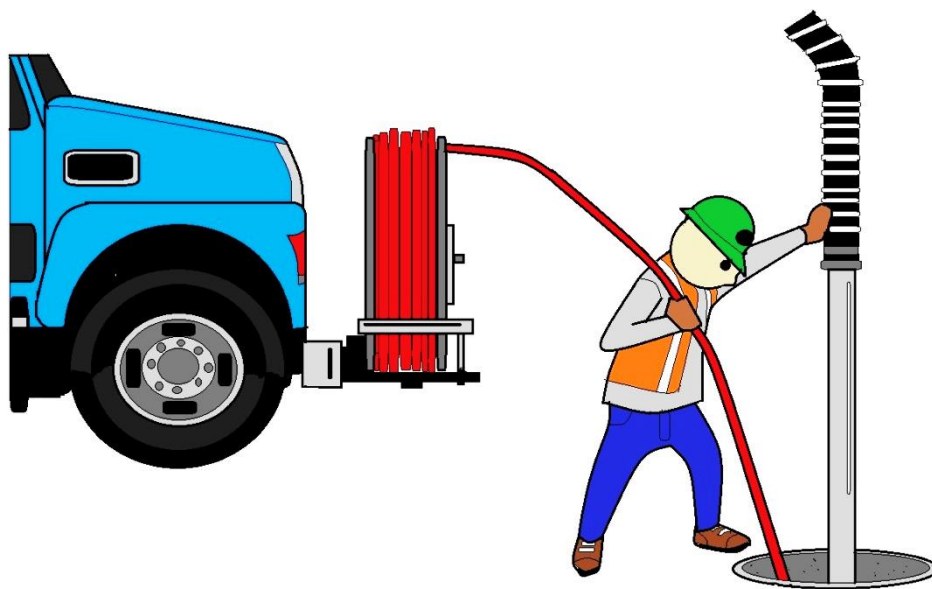
USING A VACUUM TRUCK TO CLEAN SEWER
