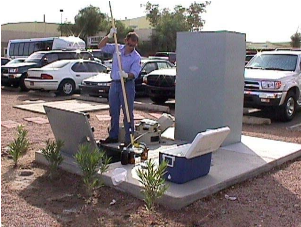
A Pretreatment Inspector sampling an SIU Interceptor. A position in Pretreatment or Stormwater is a great job promotion for any Collection System's Operator.
