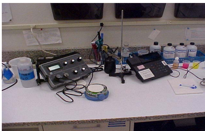
Normal wastewater sampling or pretreatment equipment found in a regulated industry. pH, ORP and Temperature measuring equipment.
