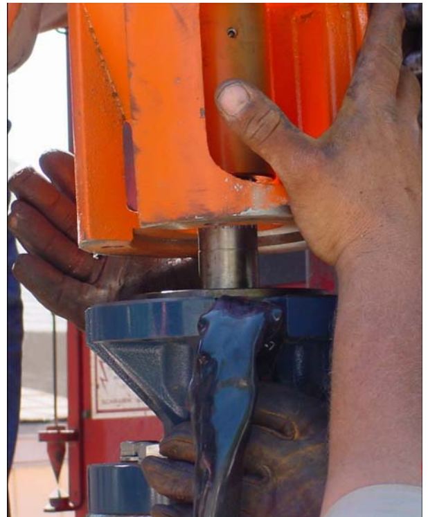
Insertion of motor spline into pump keyway
