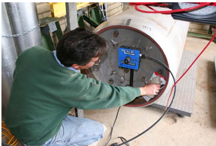
Checking for leaks with Ammonia.
