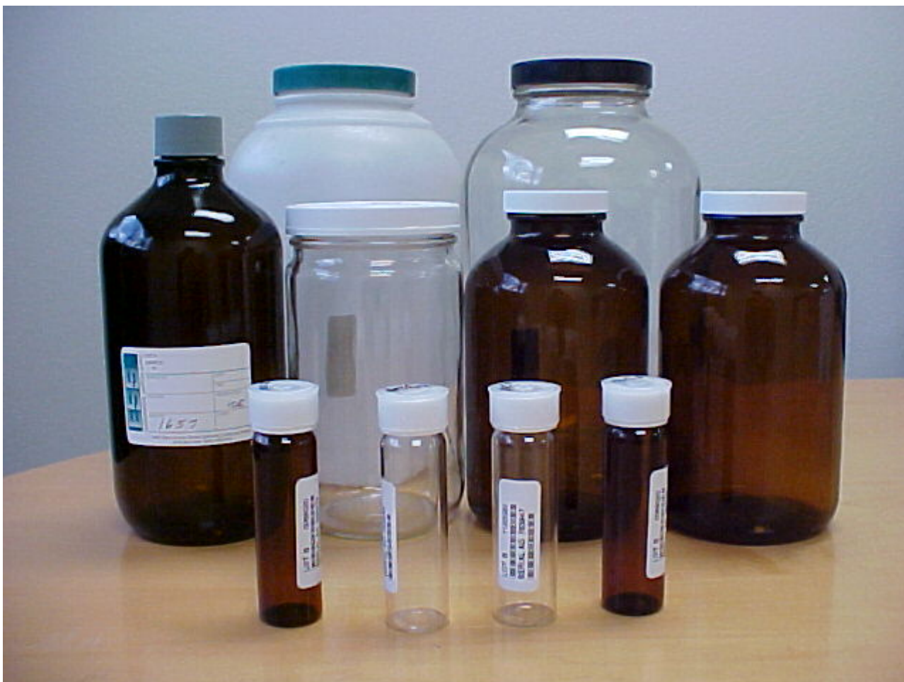
Common water sampling bottles, VOC and THM bottles are in the front.
