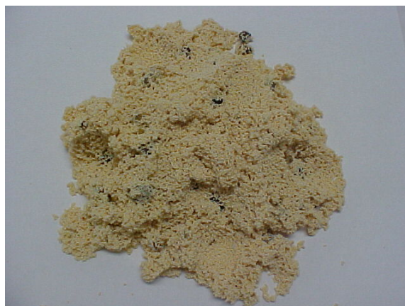
Resin beads with small stones from a nearby water well
