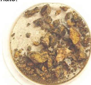
Large Rust Particles
