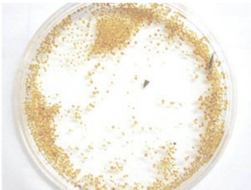
Zeolite Particles from a Water Softener
