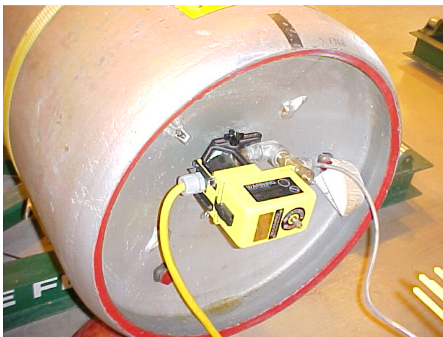
1 Ton Chlorine container with an automatic leak detection and shut-off device
