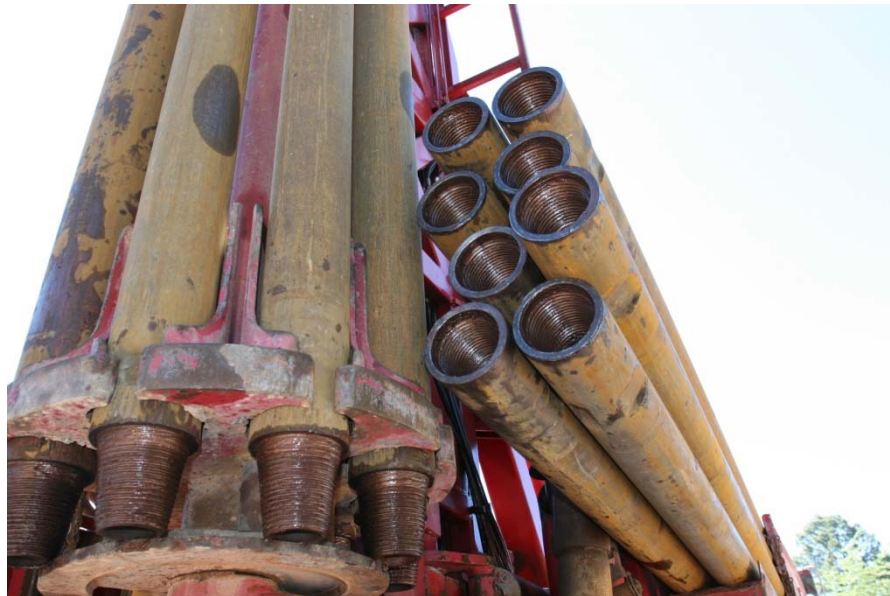
Top, drill rigging mast. Below, drilling rods on carousel and rack, notice copper pipe thread coating which prevents thread lock during high torque.
