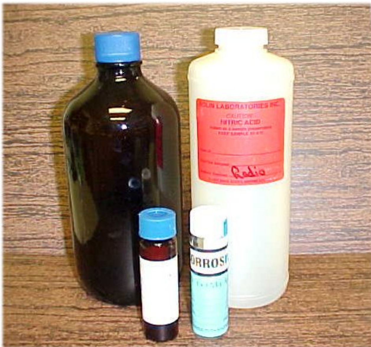
Common Sample bottles, Radiochems, VOCs, (Volatile Organic Compounds), TTHMs, Total Trihalomethanes), Nitrate, Nitrite .
