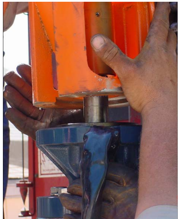
Insertion of motor spline into pump keyway
