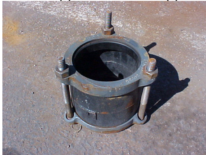
Flex Coupling used to join pipes or to “cut-in a valve”
