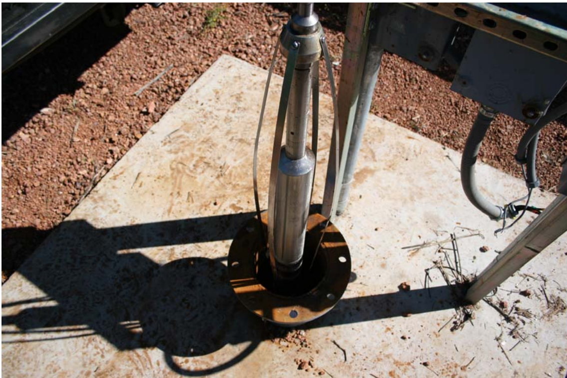
A special camera that is used to record the condition of a groundwater well.
