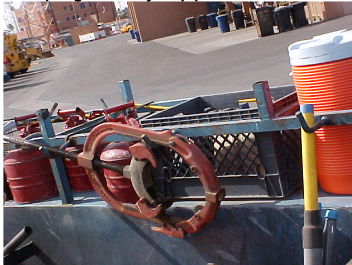
Four-Way Pipe cutting tool used for iron pipe
