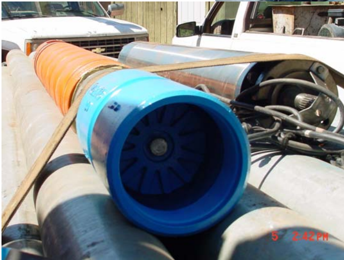
Large Diameter Submersible Pump, Motor and Column Pipe
