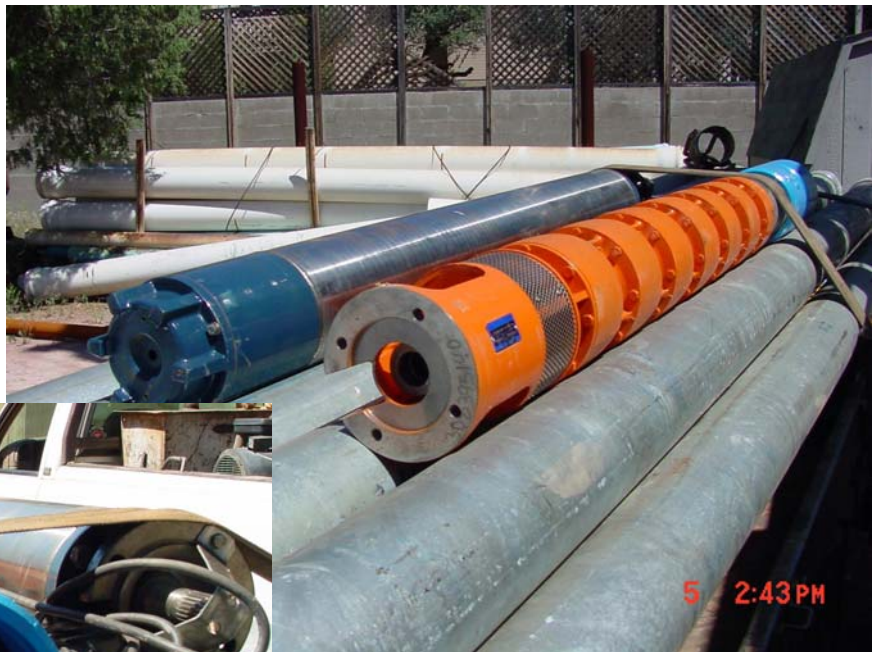
Large Diameter Submersible Pump, Motor and Column Pipe
