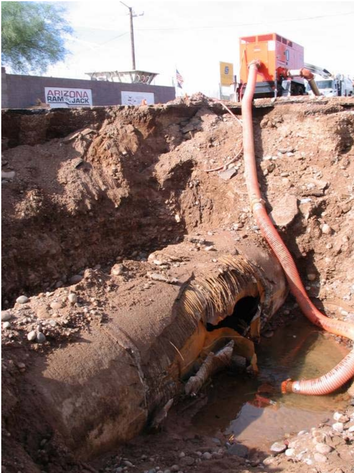
A 36 inch water main that blew out and destroyed an entire building.
