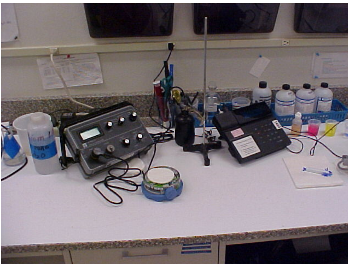
Conductivity, temperature and pH measuring equipment.
