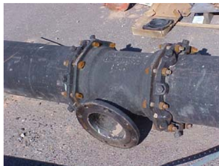
Notice the type of pipe connection device. This is known as a "Restraining Flange".
