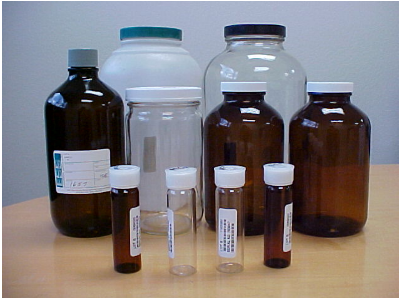
Common water sampling bottles VOC bottles are the smaller, thin bottles with the septum tops.
