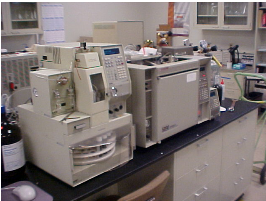
Gas Chromatograph (GC) Separates vaporized sample into individual components.
