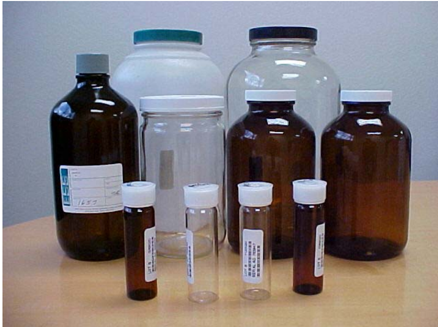
Above, 625/608, 1657, TTO/Organics, TPH/Oil/Grease Smaller bottles-TOCs, VOCs, 601/602 and 502.2.
