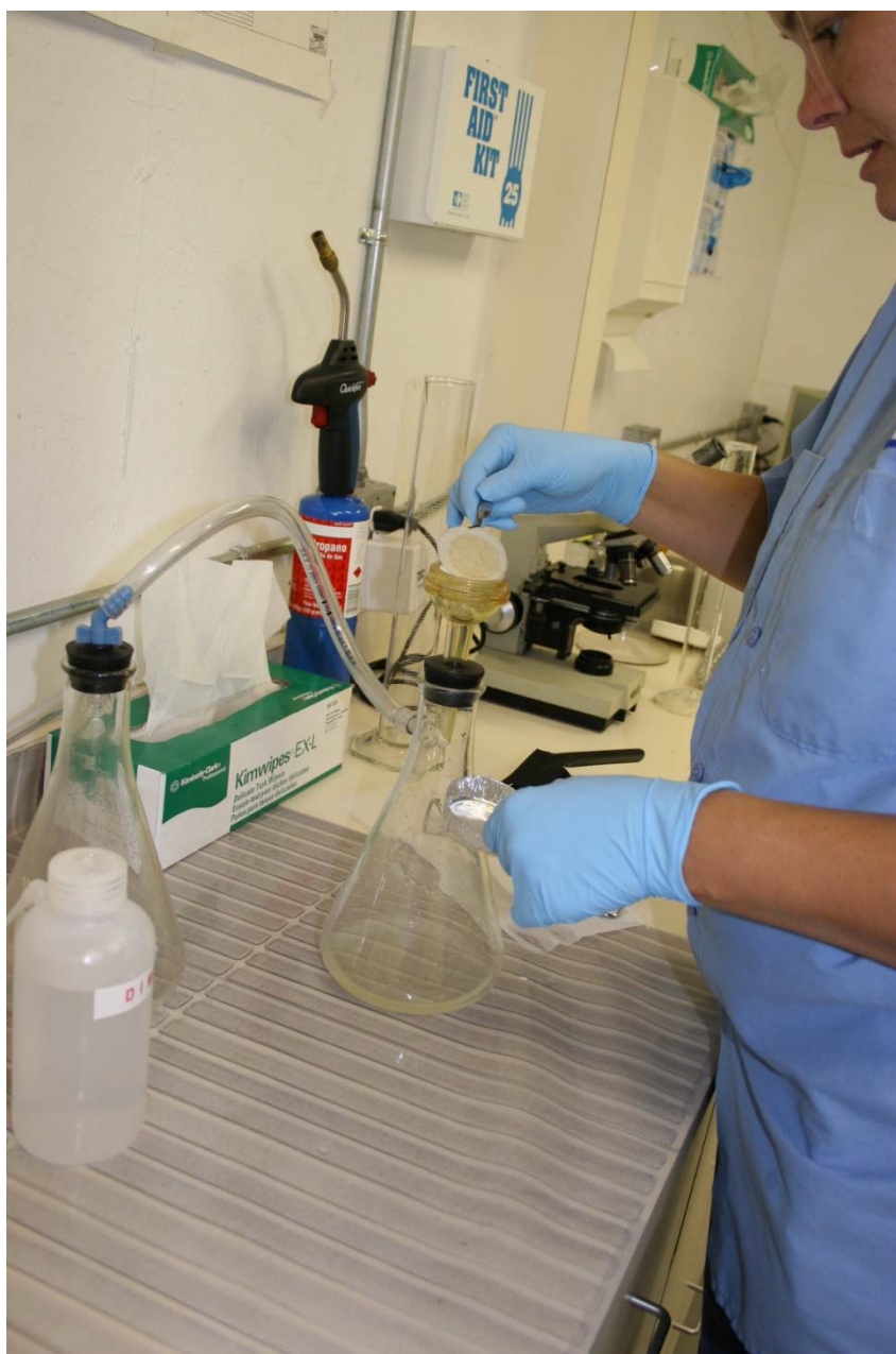
Lab tech removing filter for TSS analysis.
