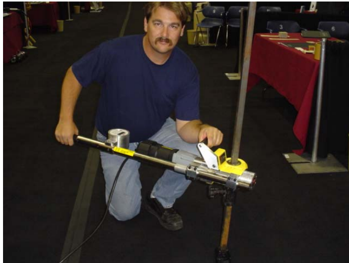
Portable valve exercising machine.
