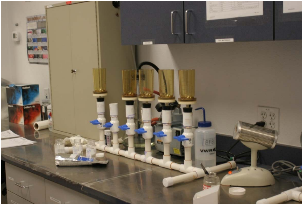
Top Photo: Analytical funnels are 100 ml filtration units that allow the membrane to be removed.
