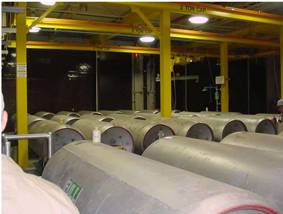
1-ton chlorine gas containers.
