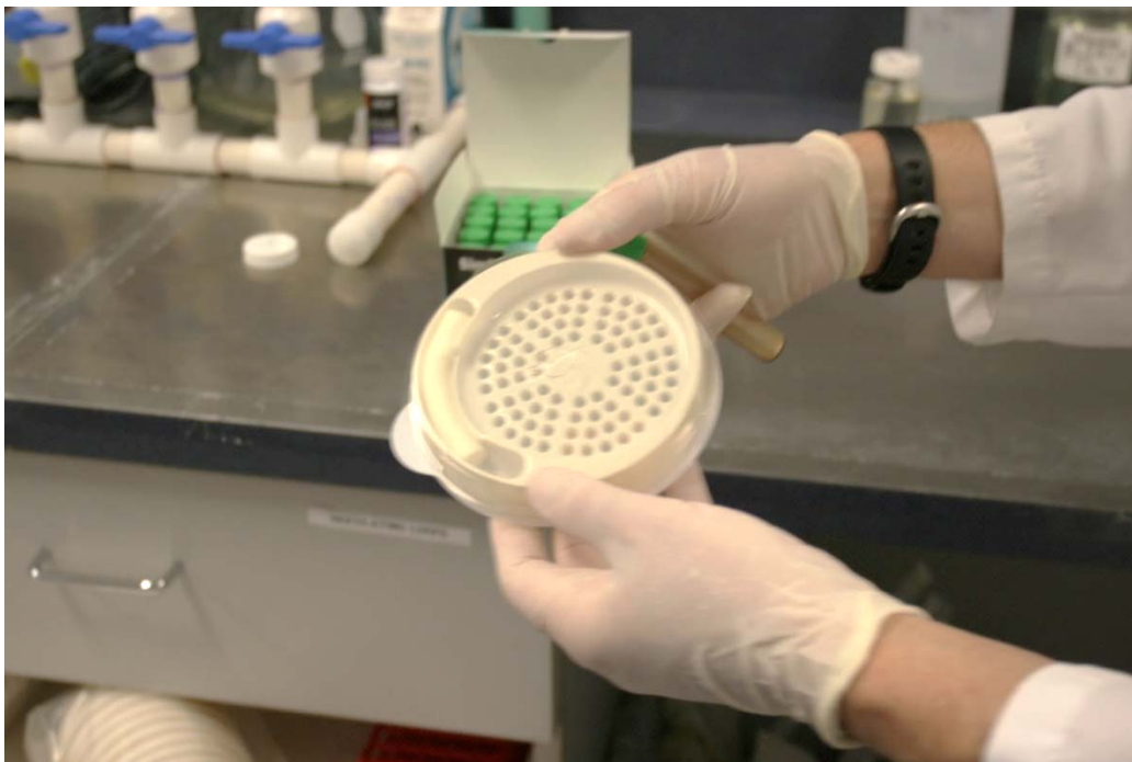
Bottom Photo: The heterotrophic plate count (HPC) is a procedure for estimating the number of live heterotrophic bacteria (requiring organic compounds of carbon and nitrogen for nourishment) in water. The technician will count the colored holes for the results.
