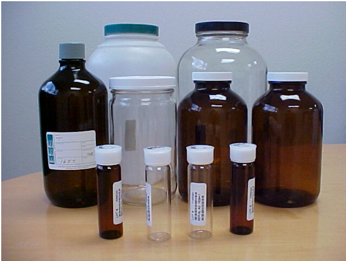
Common water sampling bottles, VOC and THM are in the front. Bacteria sample bottles are not shown.
