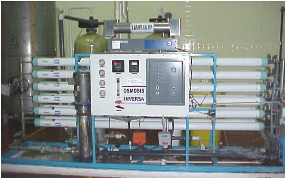
Packaged skid with instrumentation, UV, and softening.
