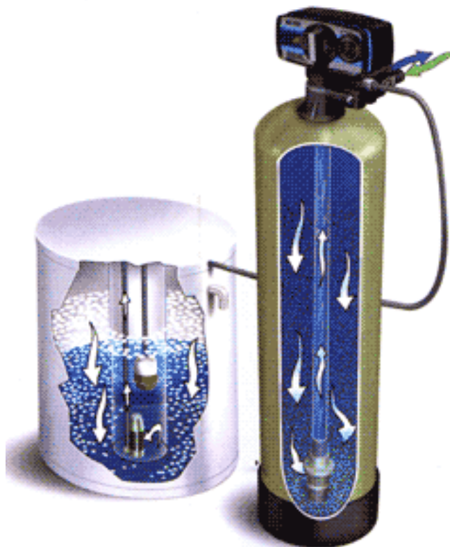
Operation of a household water softener
