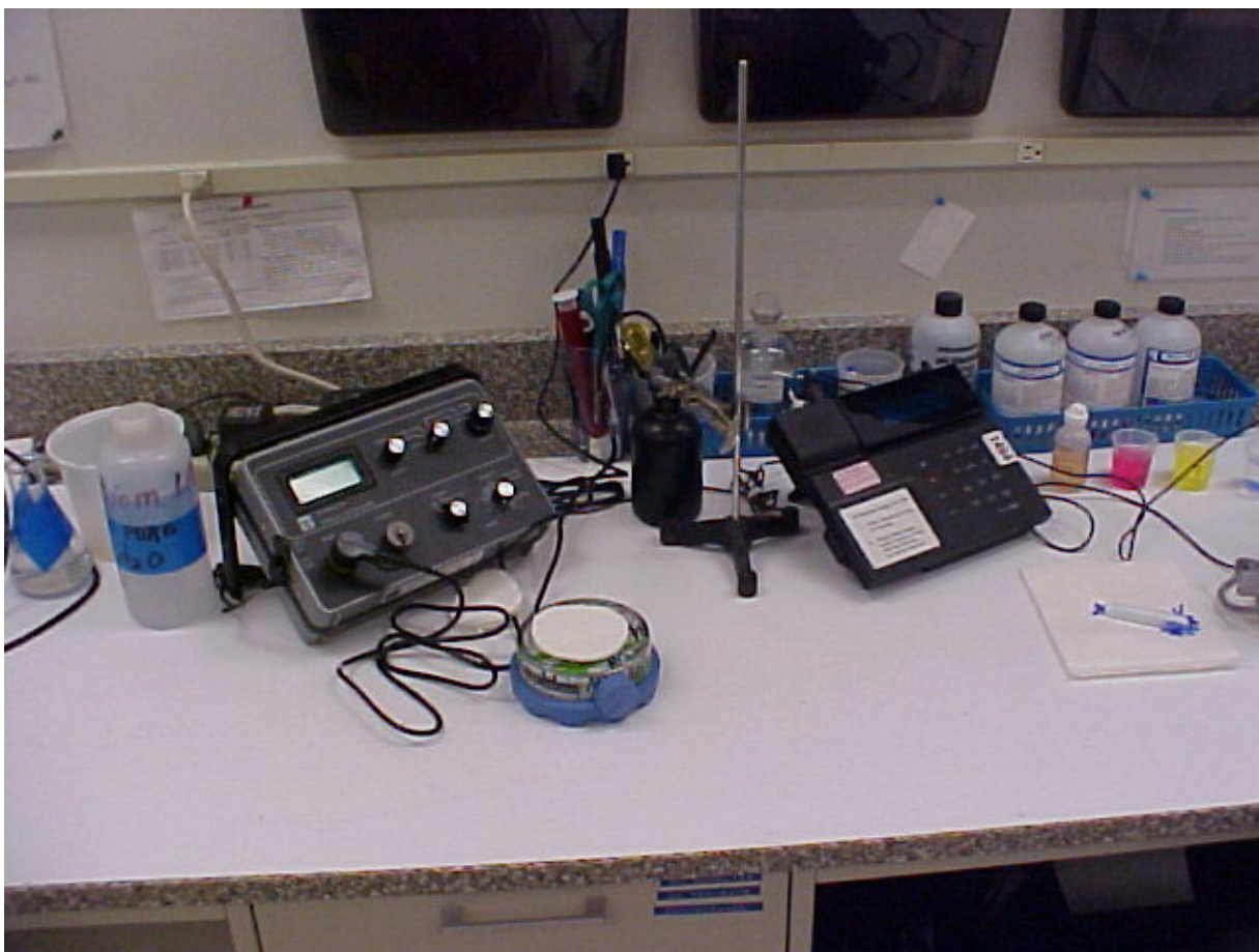
Conductivity, temperature and pH measuring equipment.
