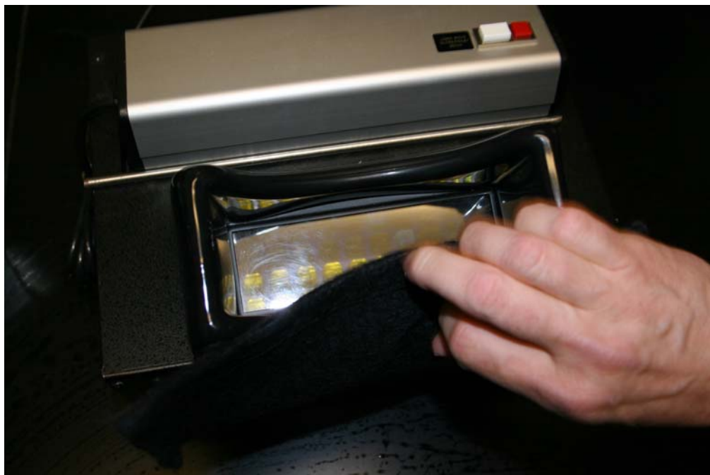
Using a black light to see fecal coliform bacteria
