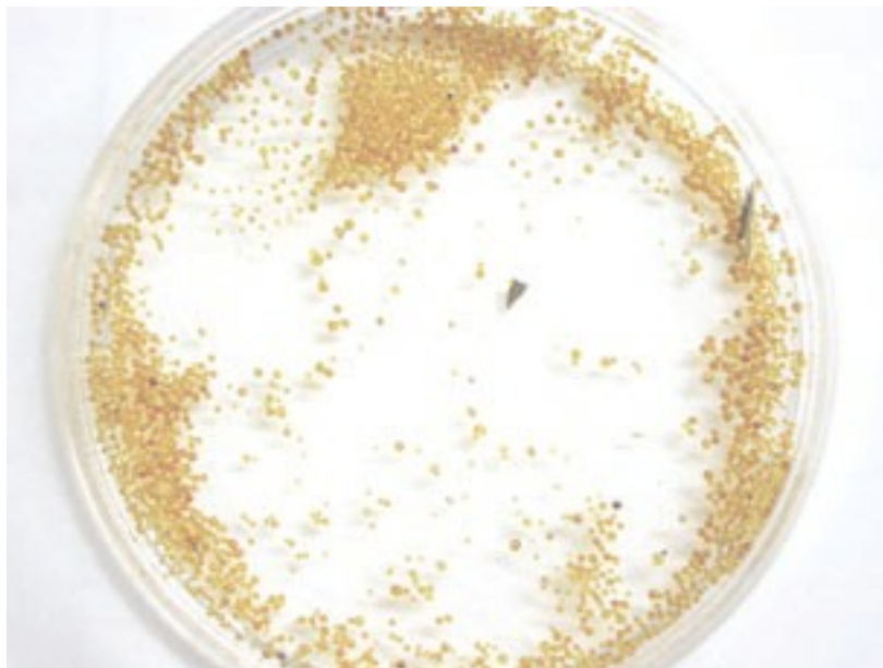
Zeolite Particles from a Water Softener
