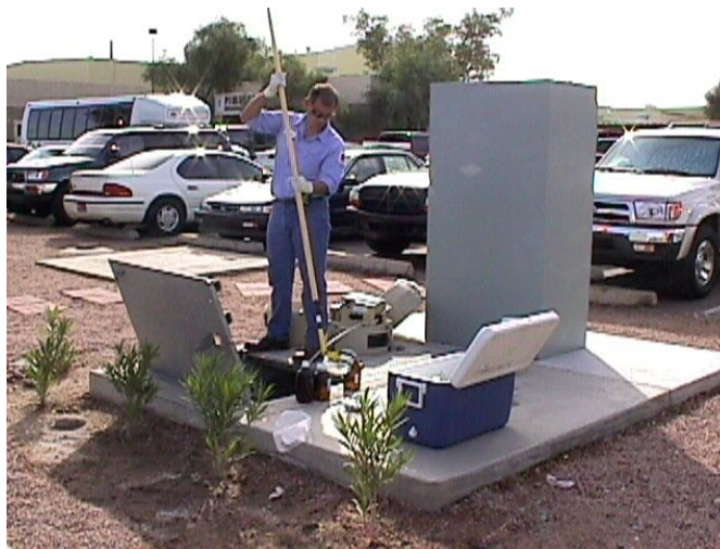
Using a pole with a sample attachment to grab a sample.
