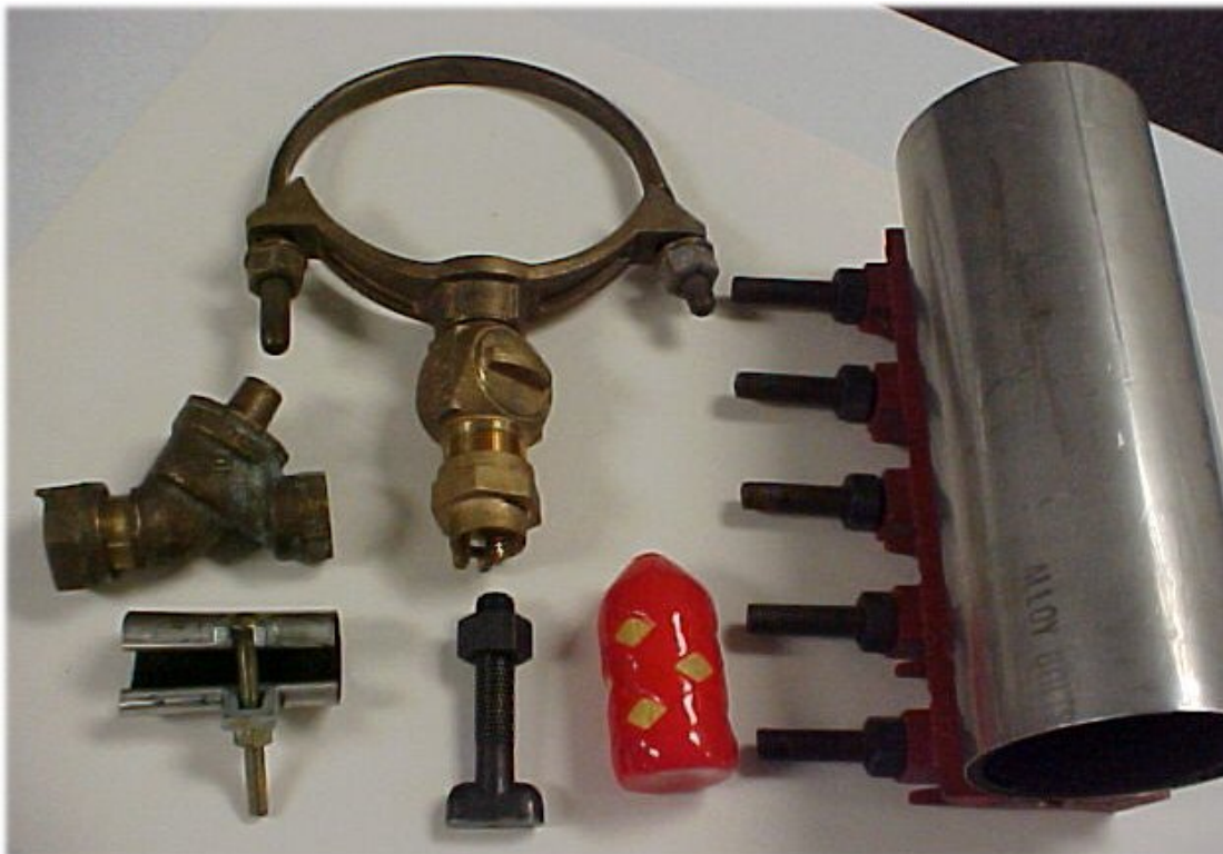
Common distribution fittings. Single check, Poly Pig, 1 inch repair clamp, 4 inch full circle clamp, T- Bolt and a corp. and saddle
