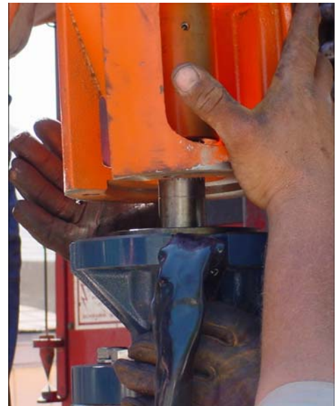
Insertion of motor spline into pump keyway
