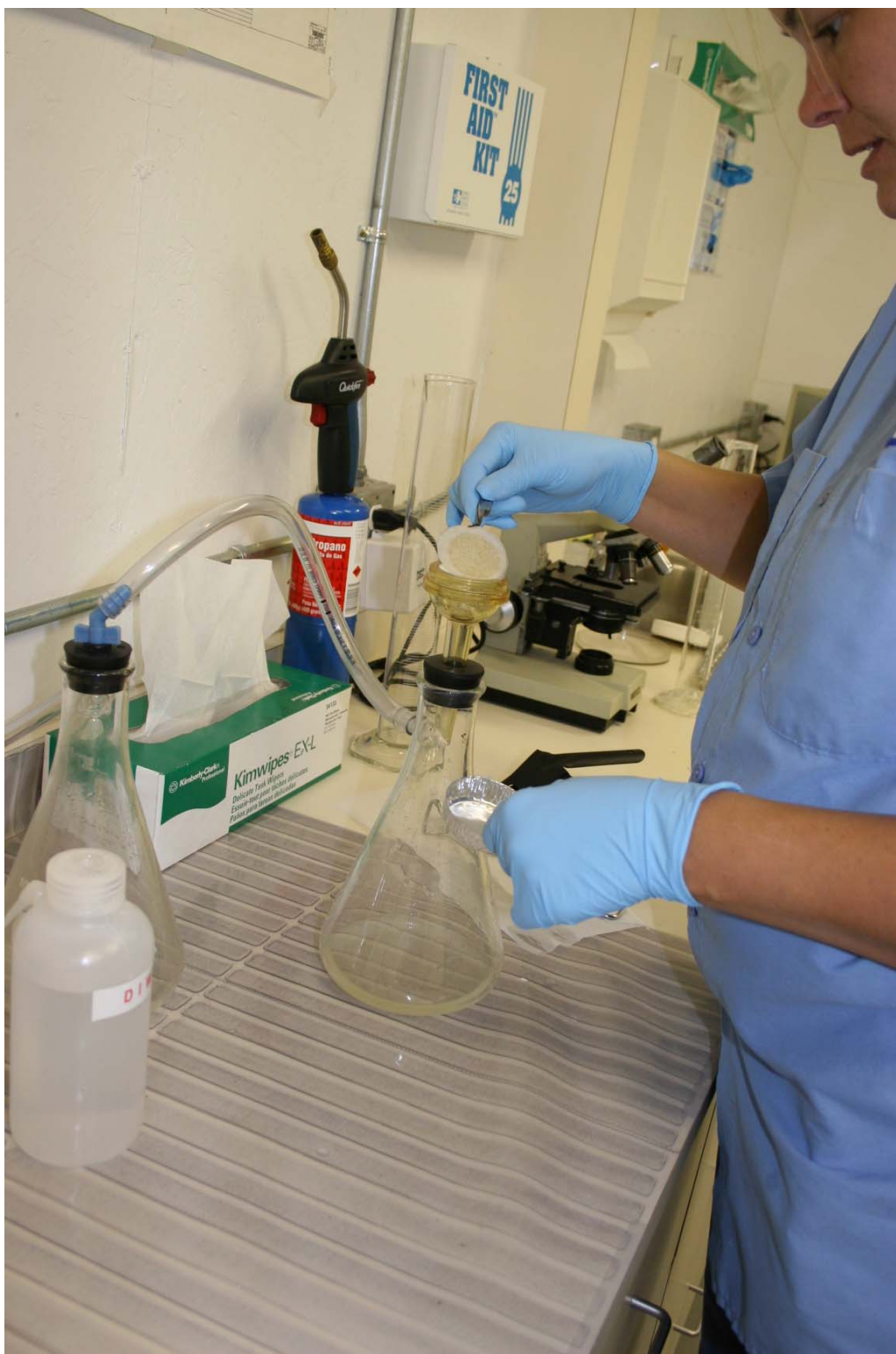
Lab tech removing filter for TSS analysis.
