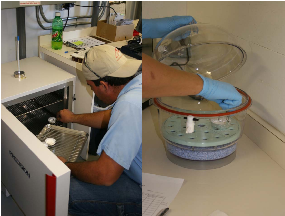
Top left, filters being baked at 105°C. Right photograph, filters in desiccant. Bottom photograph, preparation for the fecal test.
