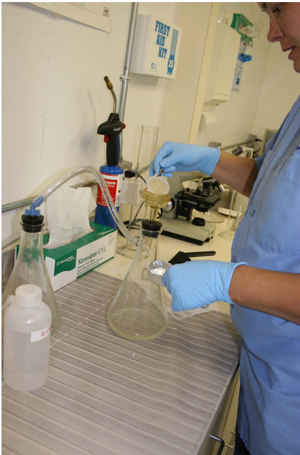
Lab tech removing filter for TSS analysis.
