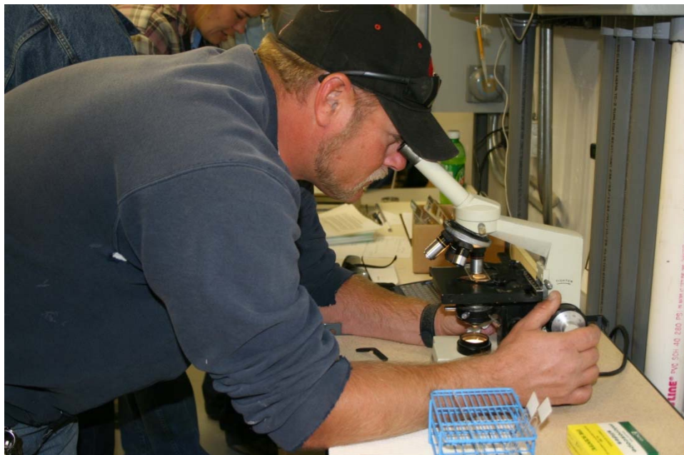
Microscopic identification is essential for any activated sludge process.
