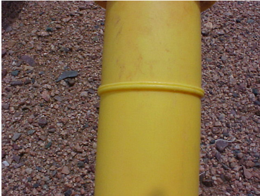
Fusion Butt Joint on plastic pipe Mechanical (compression) joint on plastic
