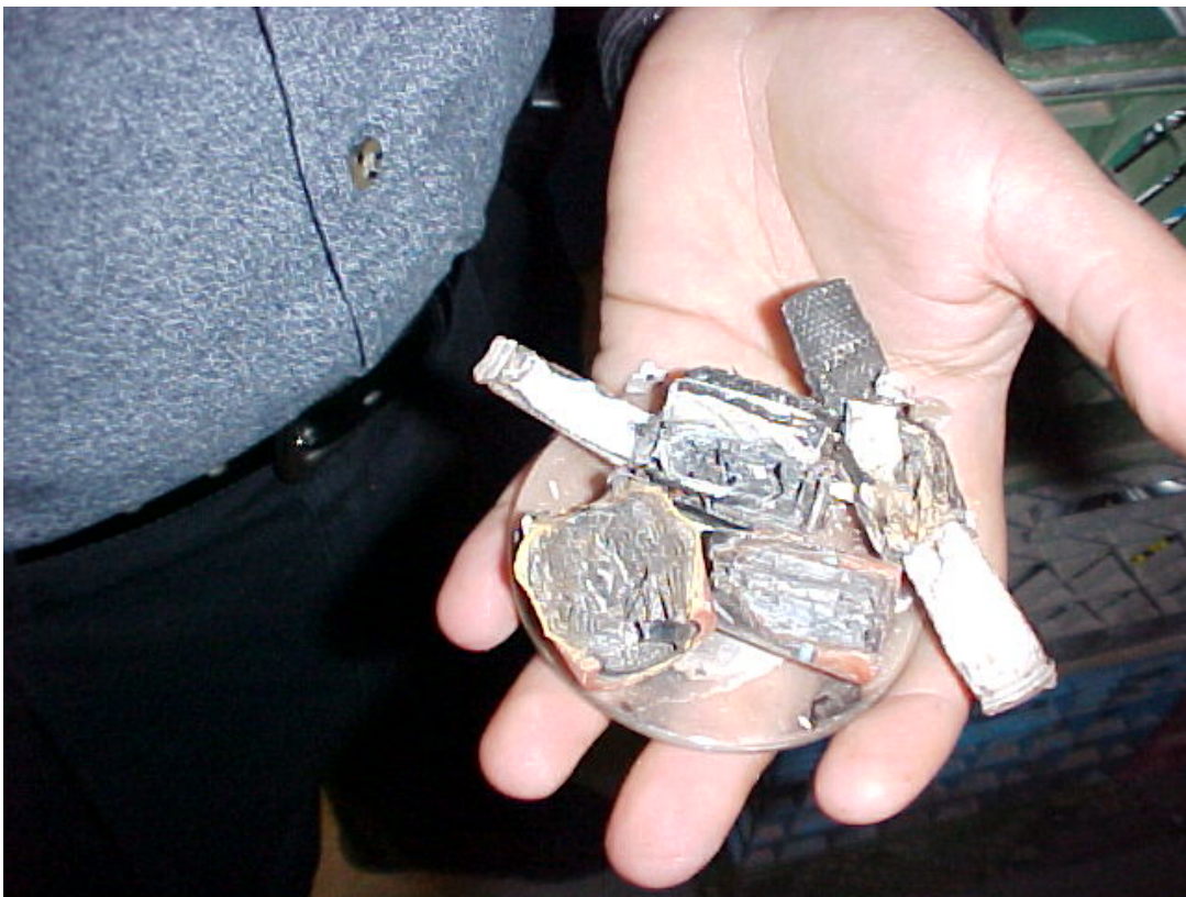
Battery Separation, Below is the effects of water and Lithium a small explosion
