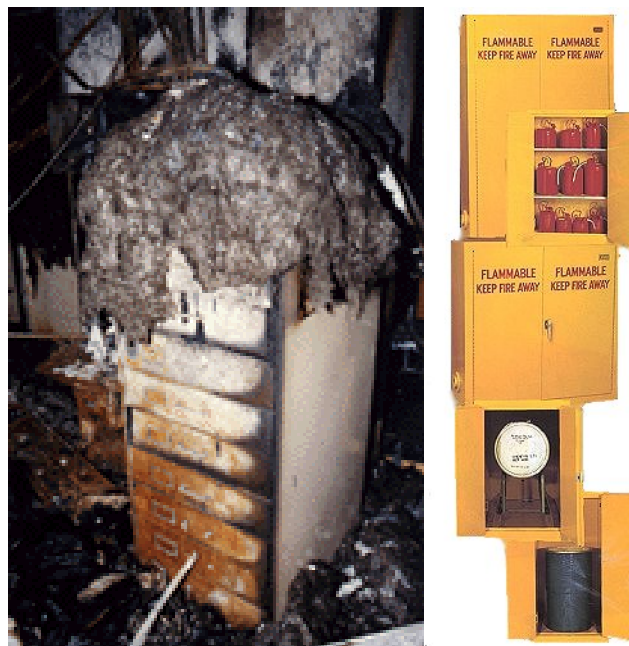
Fire Resistant File Cabinet that is burned completely and modern flammable liquids storage cabinets
