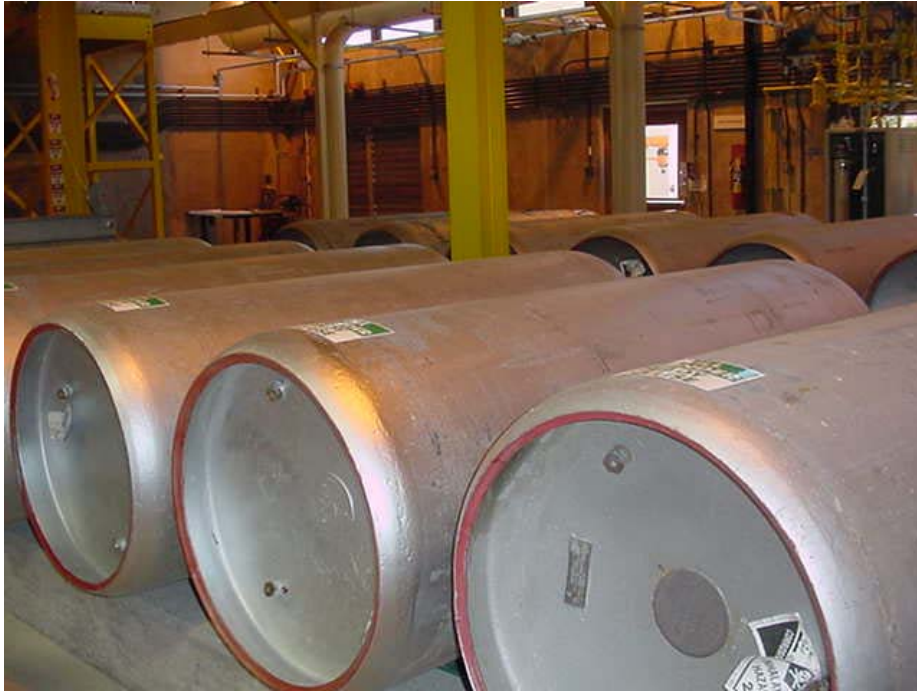
1-ton chlorine containers, rear side of container.
