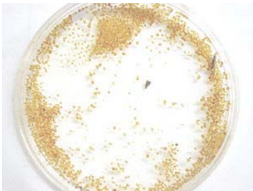
Zeolite Particles from a Water Softener.
