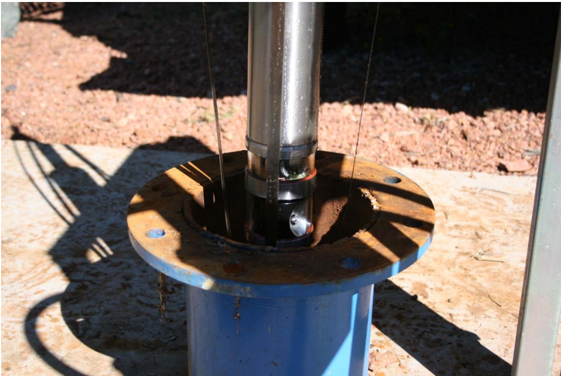
Using a video camera to see inside a groundwater well.
