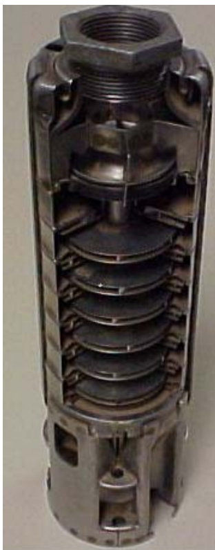
Cut away of a small submersible pump.
