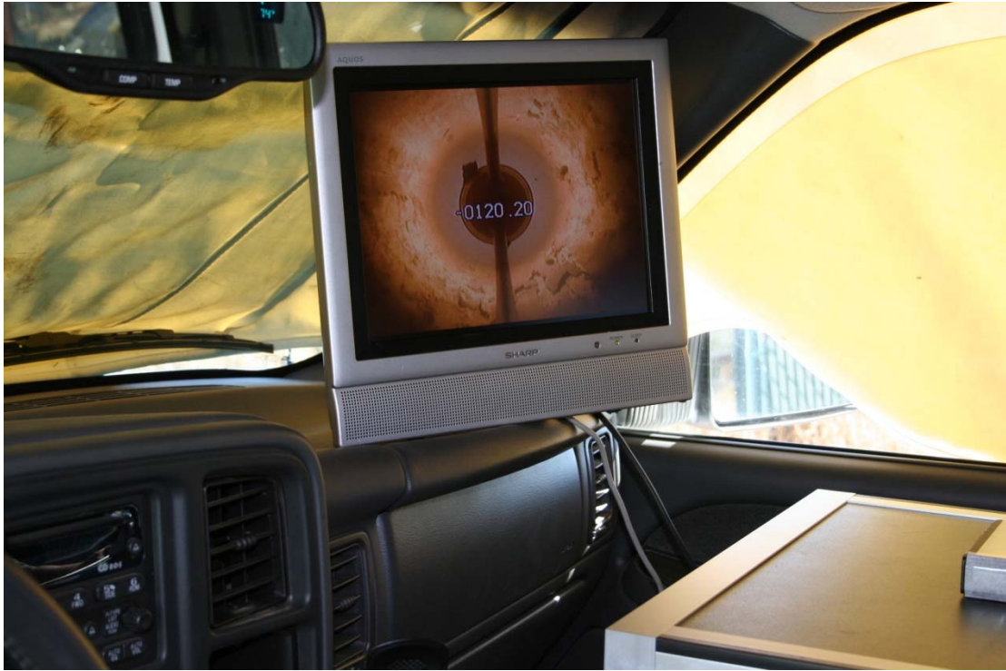
Using a video camera to see inside a groundwater well.
