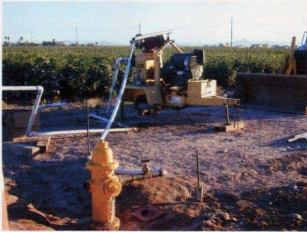
Direct connection from hydrant to pump.
