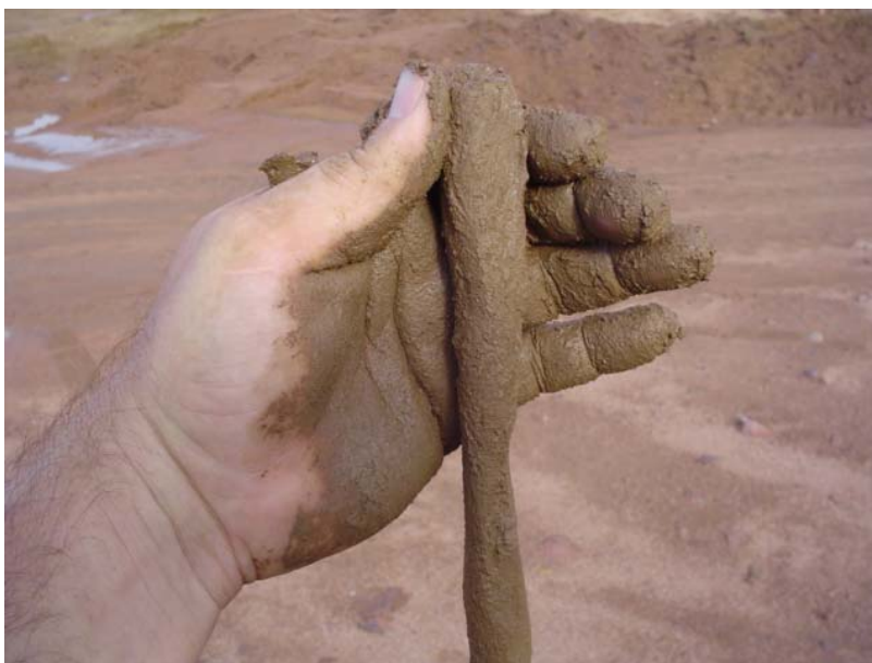
Ribbon Soil Test
