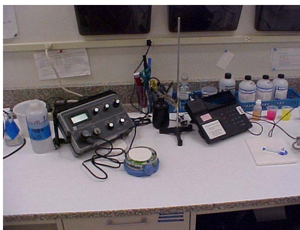
Normal wastewater sampling or pretreatment equipment found in a regulated industry. pH, ORP and Temperature measuring equipment.
