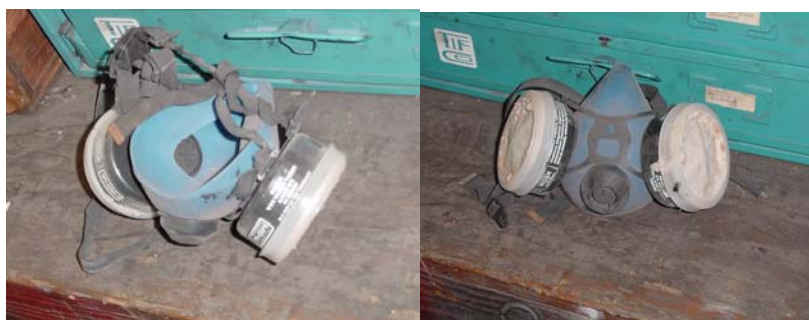
Unacceptable maintenance and storage (OSHA Violation).
