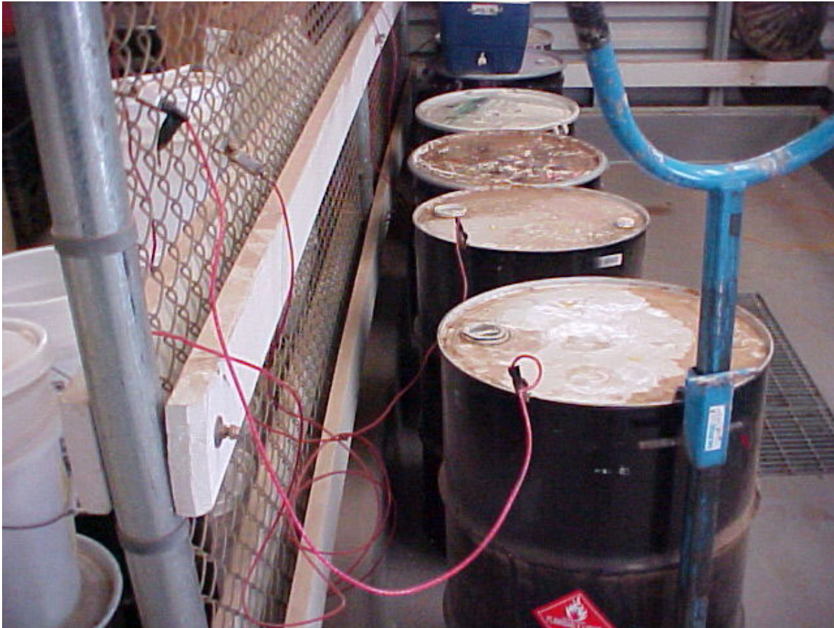
Grounded flammable drums, grounding is essential for all flammable fluids.
