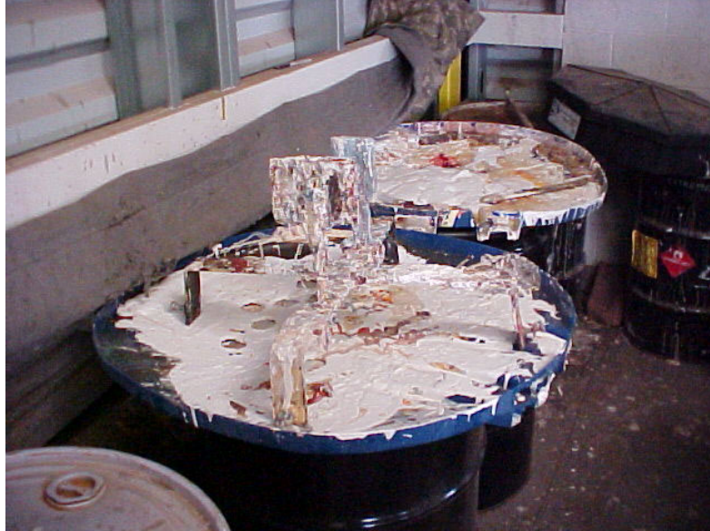
Paint drainage area with scrapers for sludge removal.
