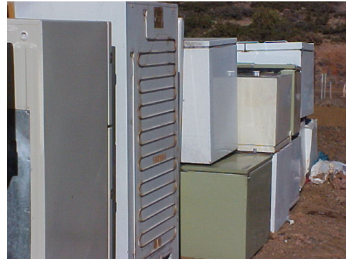
The Freon from these refrigerators was reclaimed and recycled. The metal will also be recycled.
