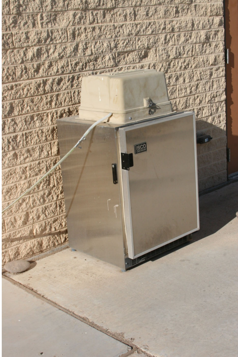
An automatic WWT sampler.
