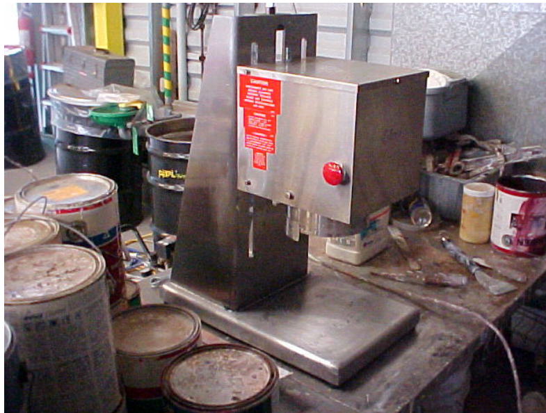
Automatic Paint Can Opener, may relive Work Related Muscle Injuries.
