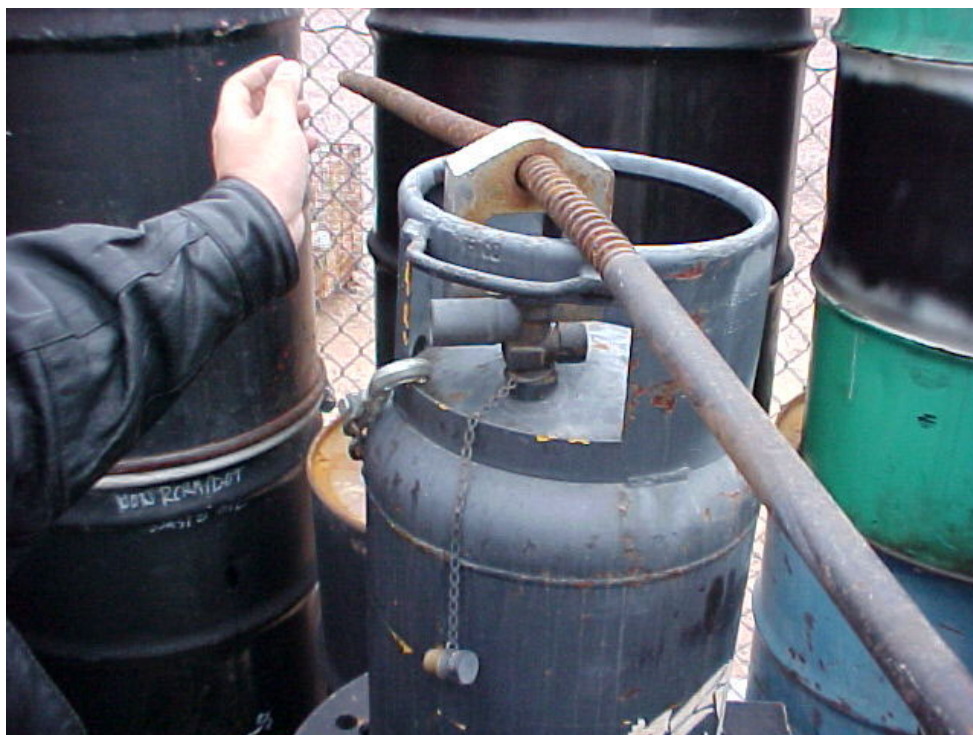
Propane tank being evacuated and later crushed for metal recycling.
