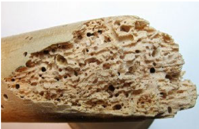
WOOD BORERS DAMAGE BASEBAT BAT
