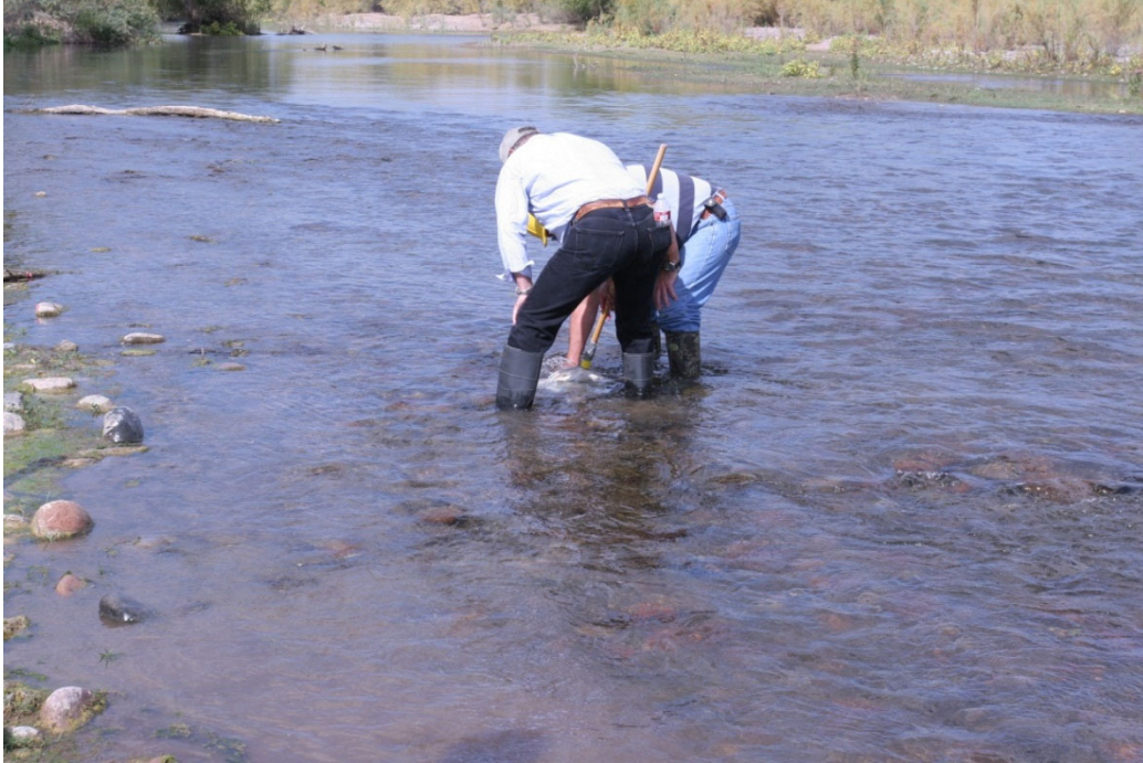
Top Photo: When sampling in the river it is suggested that a minimum of two people participate. One person is holding the collection net while the other carefully disturbs the sediment for collection.
