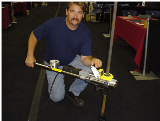
Portable valve turning-exercising machine.
