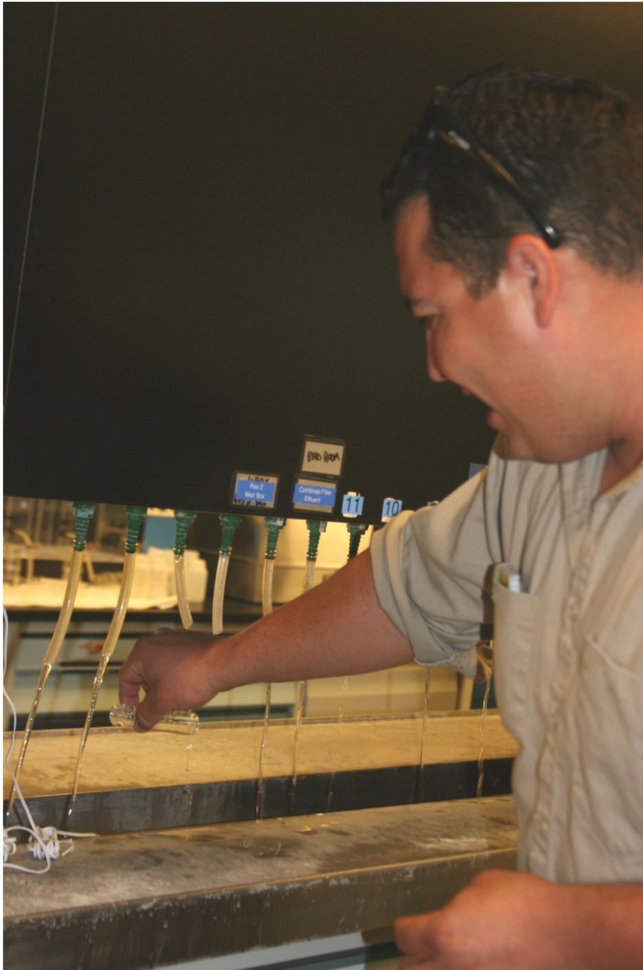
This operator is taking a grab sample to measure for turbidity.
