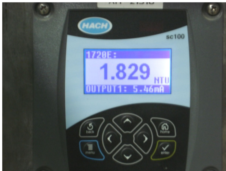
Turbidity Meter Digital Reading
