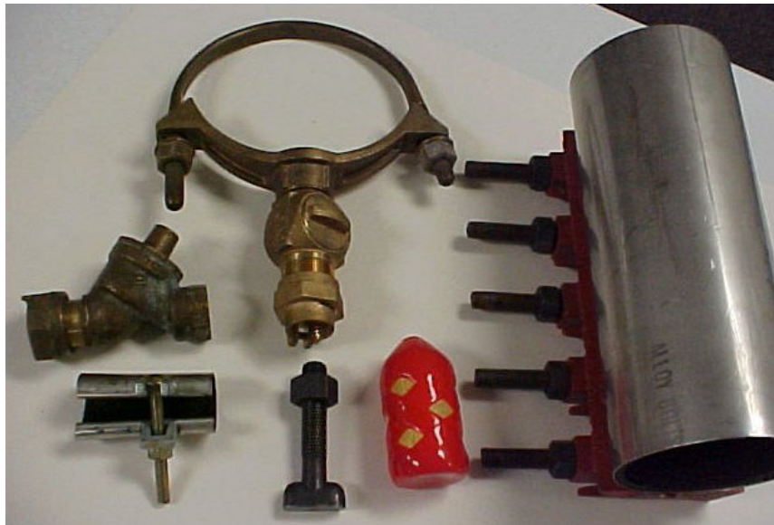
Common distribution repair fittings. Single check valve, Poly Pig, 1-inch repair clamp, 4-inch full circle clamp, T- Bolt and a corp. and saddle.
