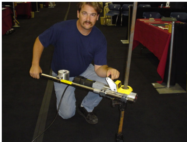
Portable valve turning-exercising machine.
