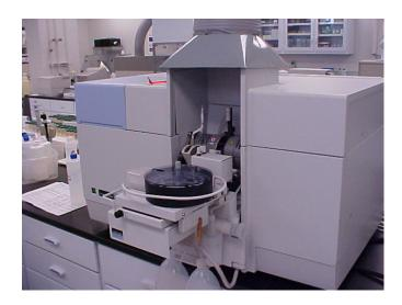
Gas Chromatograph Used for micro-contaminant water analysis.
