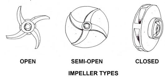
The impellers all cause a flow from the eye of the impeller to the outside of the impeller. These impellers cause what is called radial flow, and they can be referred to as radial flow impellers.
