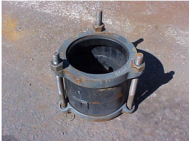
Flex Coupling-sometimes referred to as a Dayton-used to join pipes or to “cut-in a valve”. You will learn that you can use different sizes to join pipe or even file out the inside diameter to adjust to larger pipes like ACP. This flex coupling only has three bolts. I like four or more for work with larger pipes.
