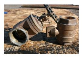
Debris allowed to remain in the pipeline (such as weld spatters, welding rods, bricks, tools, etc.) can damage the valve. After installation, cycle the valve a minimum of three times and re-torque bolts as required. Ensure that the valve is in the open position and the inside of the body bore of the valve body/body end is coated with a suitable spatter guard.
