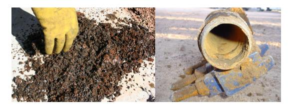
Rust and debris from cleaning a steel main.
