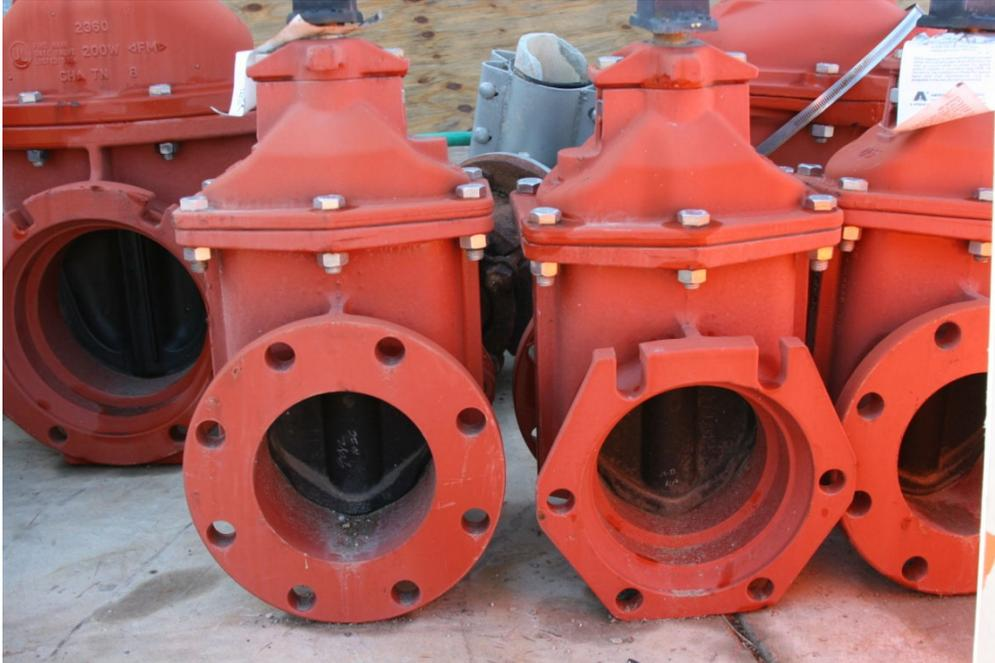
Gate valve storage procedures: Always store a gate valve with the gate up or opened. Not like in this picture. Sunlight destroy the rubber. It is best to keep the valves covered, open position and clean.
