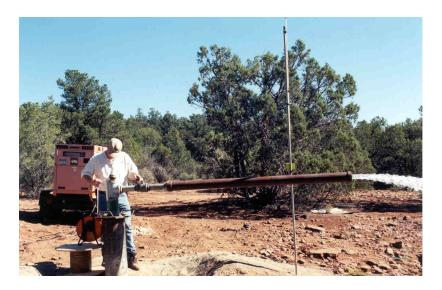
Well pumping test being conducted in photograph above. (Notice the portable electric generator for powering the pump. The Hydrogeologist is using a depth probe to measure the drop in the static water level.)
