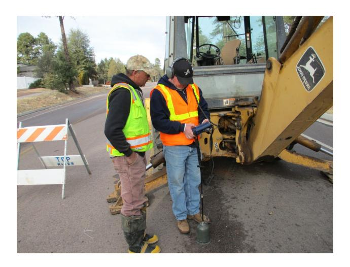
In this photograph, we see two men checking the results of a hydrophone. In areas of thick blacktop, it is difficult to locate small service leaks and slow water main breaks. A hydrophone is a microphone designed to be used underwater for recording or listening to underwater sound. Most hydrophones are based on a piezoelectric transducer that generates electricity when subjected to a pressure change.
