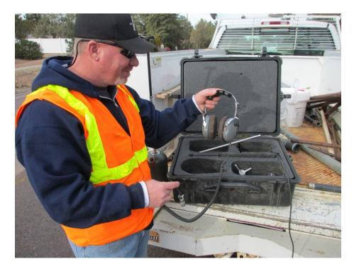
Leak detection is critical for finding difficult to locate leaks. There are many devices to choose from. All of these devices magnify the sound of the leak to pinpoint the area of damage. Plastic pipe is the most difficult and copper is the easiest to locate.
