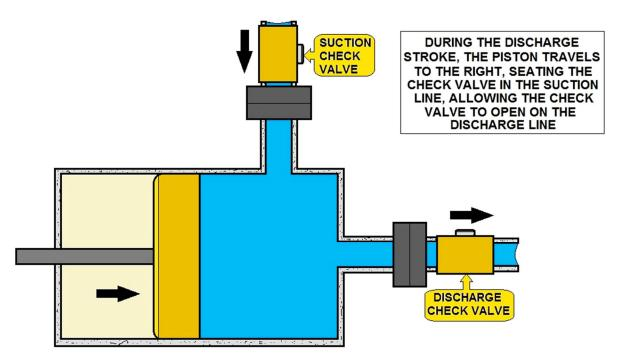
PISTON TYPE -POSITIVE DISPLACEMENT PUMP
