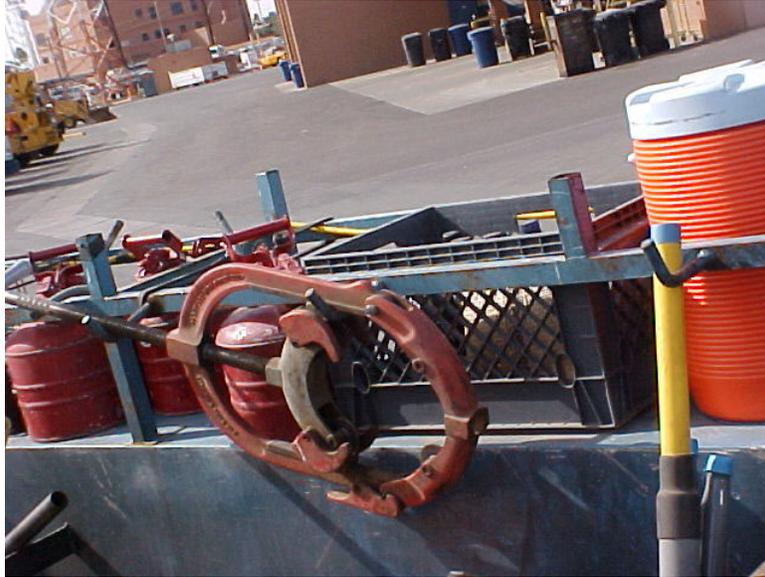
Here is a four-way pipe cutting tool used for iron pipe. Be careful not to break the wheels by over tightening. I personally like 4-Ways because of the nice cut. You will learn to recognize the distinct snap of cut pipe. The only drawback to these cutters is cutting a small section out of the main. You may need to make two or three more cuts and break the section out with a cocking hammer. It will easily cut Ductile, galvanized, and even plastic.
