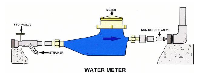
Water meters are used to measure the volume of water used by residential and commercial building that are supplied with water by a public water supply system.
