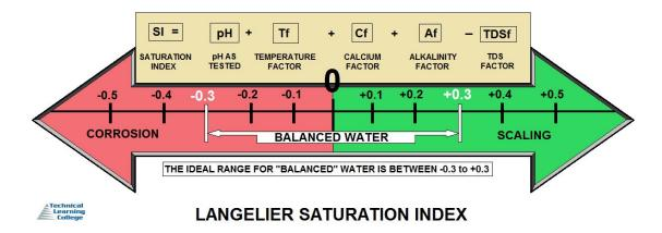
Water with a Langelier saturation index of 1.0 is one pH unit above saturation. Reducing the pH by 1 unit will bring the water into equilibrium. This occurs because the portion of total alkalinity present as  $CO_3^{2-}$  decreases as the pH decreases, according to the equilibria describing the dissociation of carbonic acid:
