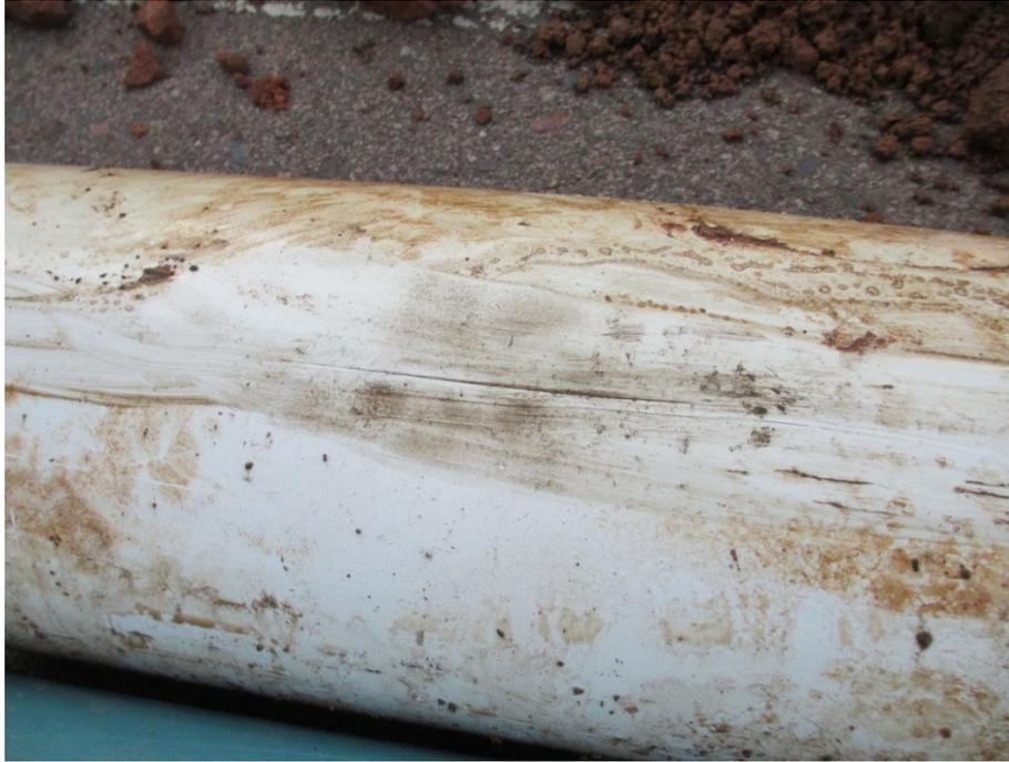
Generally speaking, water main breaks are much more intense than service leaks. This scenario with examine a hairline crack caused by poor installation. The water main was laid on a sharp rock without proper bedding. A slight water main leak is often confused with a service line leak and can be difficult to find.
