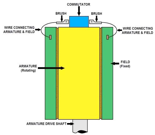
DIAGRAM SHOWING MECHANICAL CONSTRUCTION
