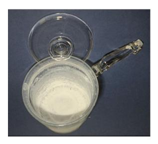
When hard water is heated, scale forms much faster. In particular, when the magnesium hardness is more than about 40 mg/l (as CaCO<sub>3</sub>), magnesium hydroxide scale will deposit in hot water heaters that are operated at normal temperatures of 140-150°F (60-66°C).
