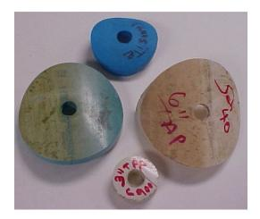
Various types and sizes of coupons or tap cut-outs. Collect and date these cut-outs to determine the condition of the pipe or measure corrosion.
