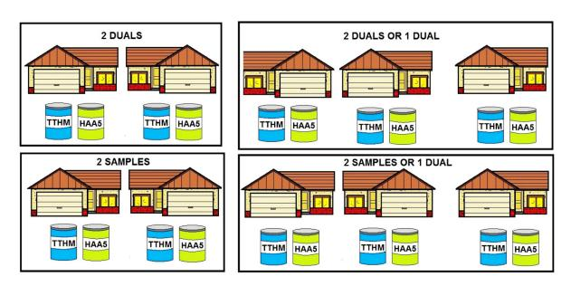
STAGE 2 DISINFECTION BYPRODUCT RULE REPEAT (TRIGGERED) SAMPLING DIAGRAM
