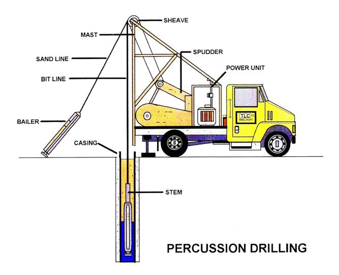
Percussion drilling is a commonly found groundwater production drilling technique in which a drill bit attached to rope or cable is repeatedly raised and lowered, impacting soil and rock and making the hole deeper. Frequently used to drill wells or during mineral prospecting activities, percussion drilling has been used for thousands of years and is adaptable to whatever technology is available.
