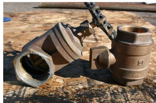
Debris allowed to remain in the pipeline (such as weld spatters, welding rods, bricks, tools, etc.) can damage the valve. After installation, cycle the valve a minimum of three times and re-torque bolts as required. Ensure that the valve is in the open position and the inside of the body bore of the valve body/body end is coated with a suitable spatter guard.
