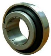
The type of material used for the seal faces will depend upon the service of the pump. Most water service pumps use a carbon material for one of the seal faces and ceramic (tungsten carbide) for the other. When the seals wear out, they are simply replaced.
