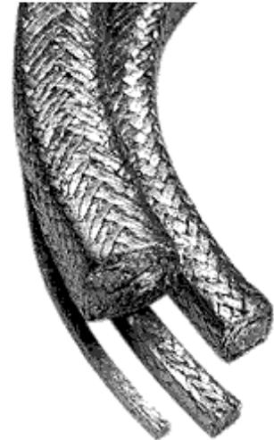
To ensure the longest possible service from pump packing, make certain the shaft or sleeve is smooth when the packing is removed from a gland. Rapid wear of the packing will be caused by roughness of the shaft sleeve (or shaft where no sleeve is installed). If the shaft is rough, it should be sent to the machine shop for a finishing cut to smooth the surface. If it is very rough, or has deep ridges in it, it will have to be renewed. It is absolutely necessary to use the correct packing.
