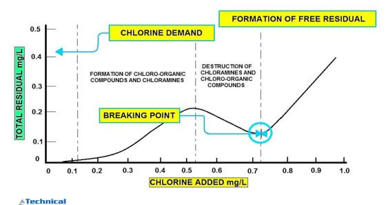
**REACTION OF CHLORINE IN WATER**
