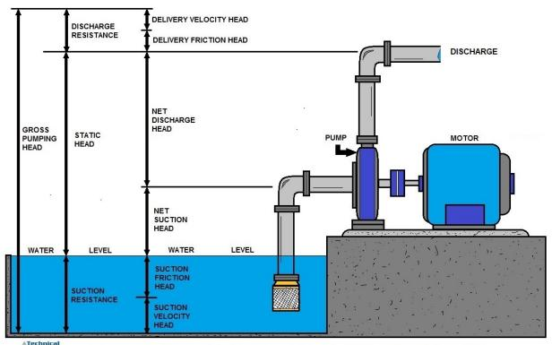
**FACTORS IN DETERMINING A TYPICAL PUMP INSTALLATION**
