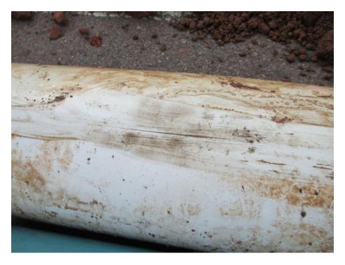
Generally speaking, water main breaks are much more intense than service leaks. This scenario with examine a hairline crack caused by poor installation. The water main was laid on a sharp rock without proper bedding. A slight water main leak is often confused with a service line leak and can be difficult to find.
