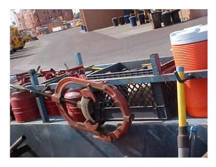
Here is a four-way pipe cutting tool used for iron pipe. Be careful not to break the wheels by over tightening. I personally like 4-Ways because of the nice cut. You will learn to recognize the distinct snap of cut pipe. The only drawback to these cutters is cutting a small section out of the main. You may need to make two or three more cuts and break the section out with a cocking hammer. It will easily cut Ductile, galvanized, and even plastic.
