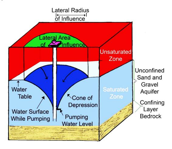
When a well is installed in an unconfined aquifer, water moves from the aquifer into the well through small holes or slits in the well casing or, in some types of wells, through the open bottom of the well. The level of the water in the well is the same as the water level in the aquifer.
