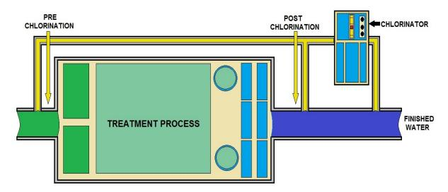
CHLORINE FLOW IN A TREATMENT PLANT
