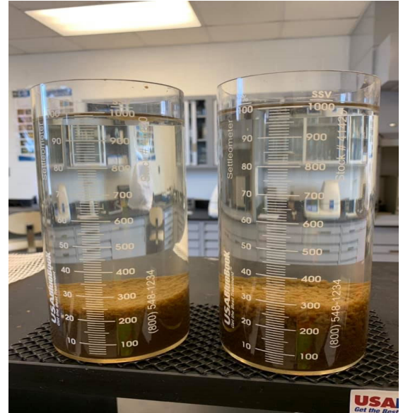
Well-settled mixed liquor with a clear supernatant
