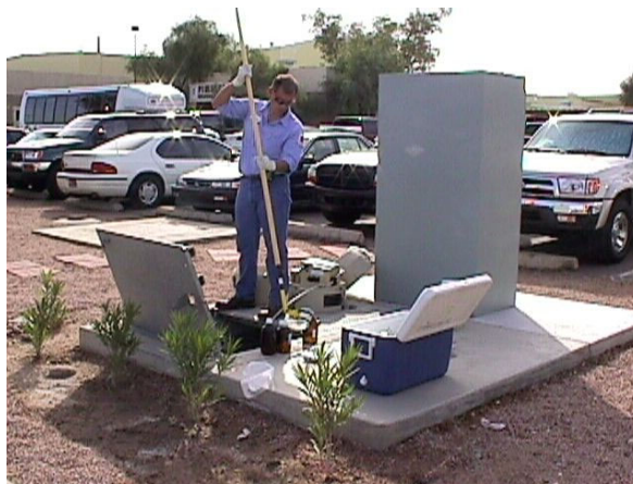
Using an extension pole with a sample attachment to grab a sample.
